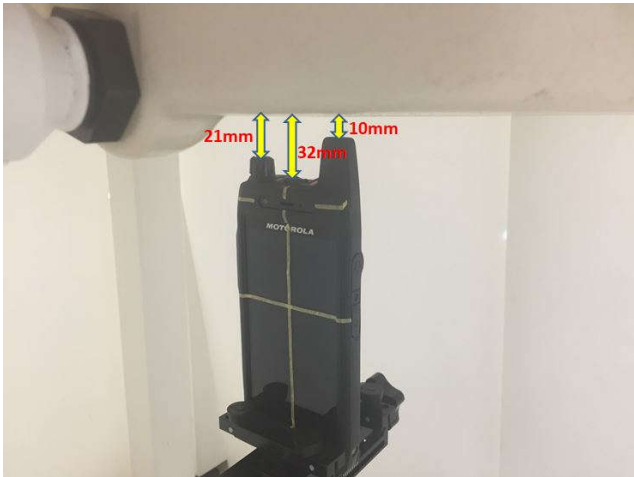
Top Side, Test Separation 10 mm
