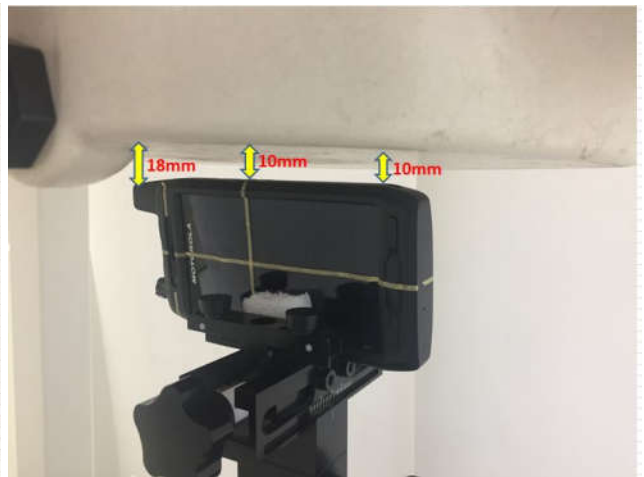
Right Side, Test Separation 10 mm
