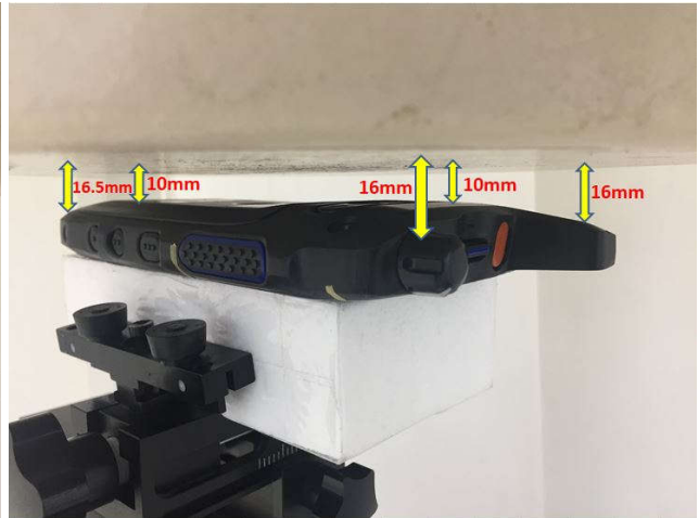
Back, Test Separation 10 mm
