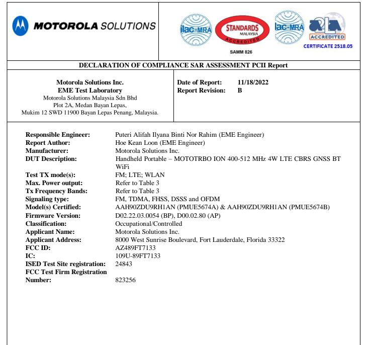
The test results clearly demonstrate compliance with FCC Occupational/Controlled RF Exposure limits of 8 W/kg averaged over 1 gram per the requirements of FCC 47 CFR § 2.1093 and RSS-102 (Issue 5).
