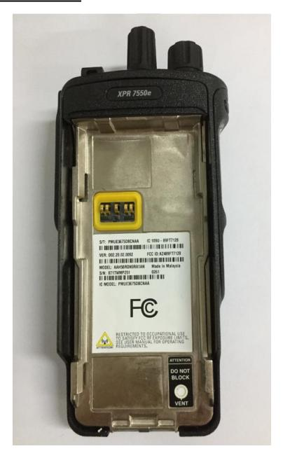
Back View for Full Keypad with Display Model (FCC/IC label location)
