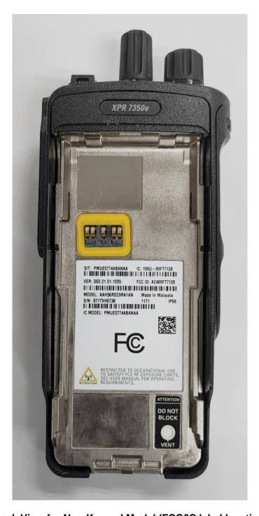
**Back View for Non Keypad Model (FCC/IC label location)**
