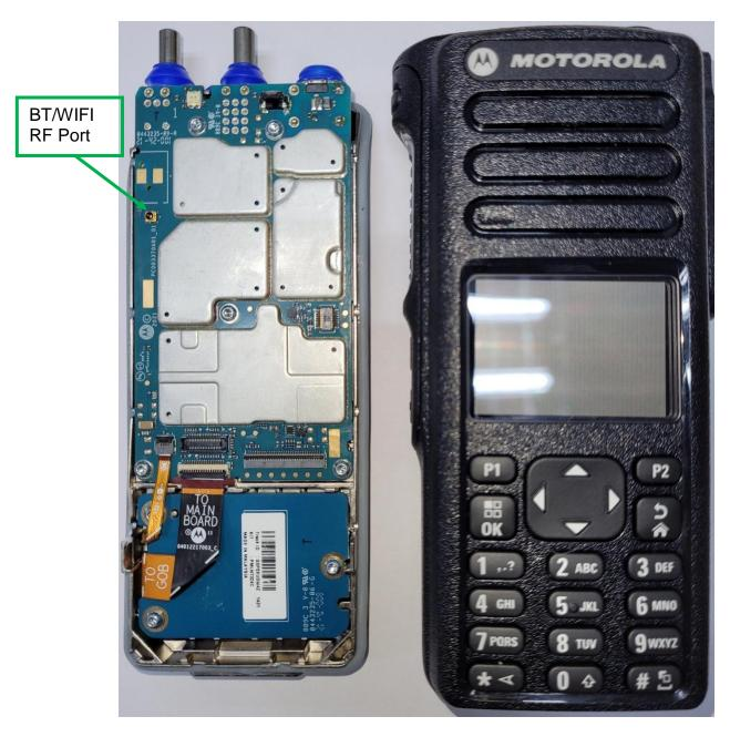
RF Board With Chassis and Housing (Front Side) FKP Non-TIA4950
