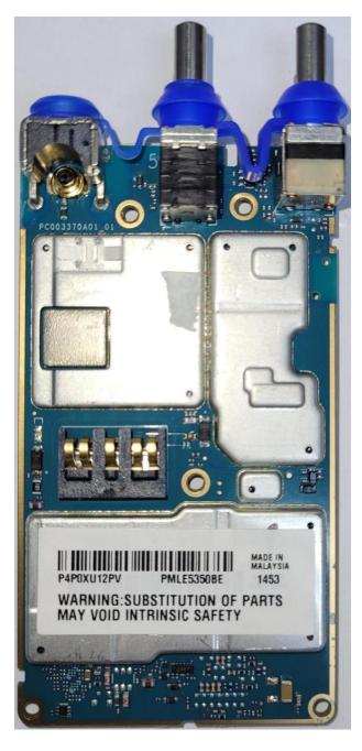
RF Board With Shields (Bottom) TIA4950
