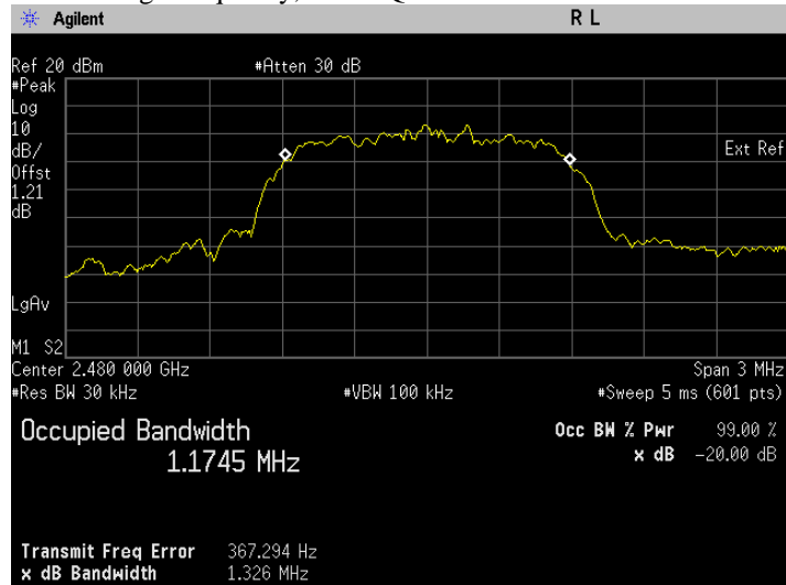
iii. The 20 dB BW & occupied bandwidth test with result at high frequency, Pi/4 DQPSK.
