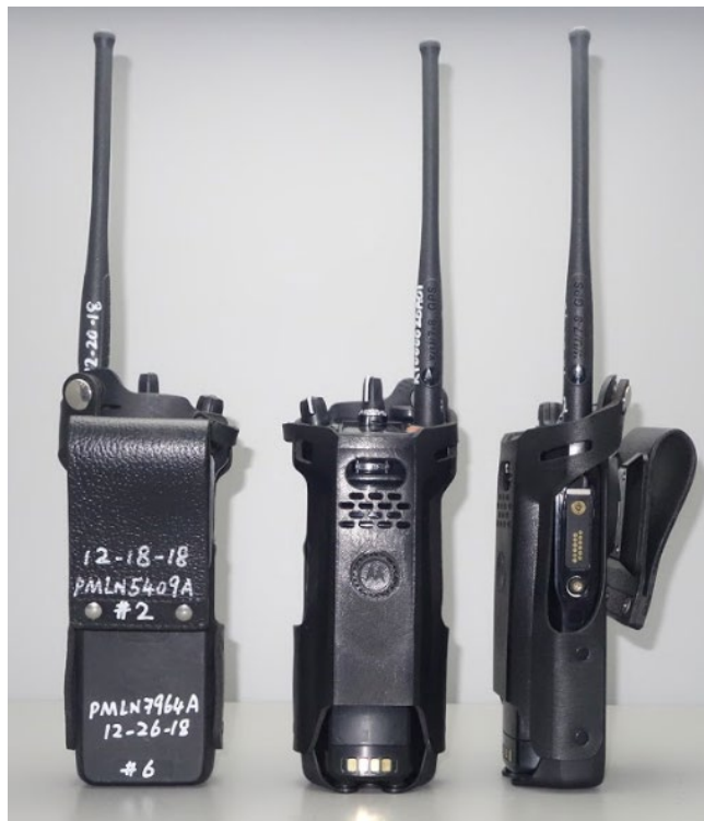
PMLN7964A with PMLN5409A (Left to Right): DUT Back view, DUT Front View, DUT Side view
