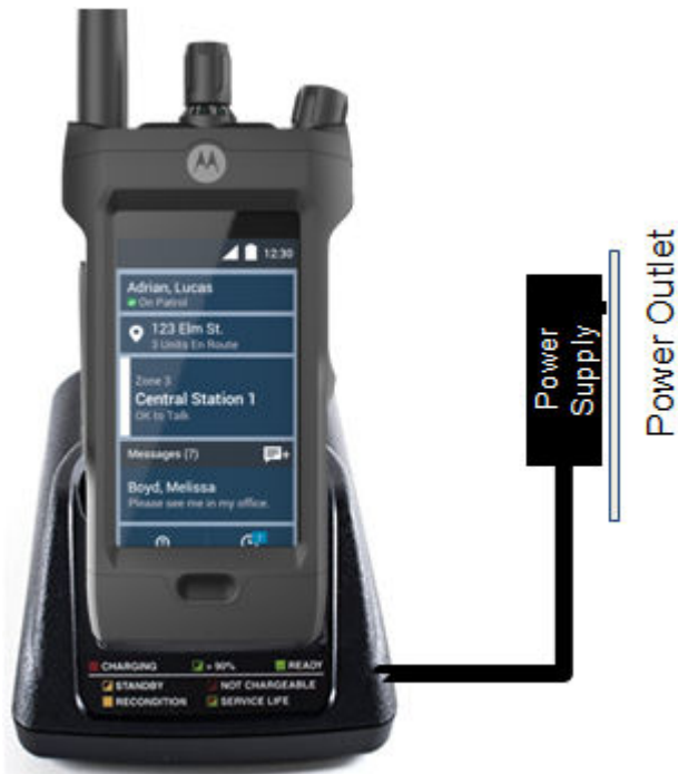
Figure 1: Charging the Radio using a Single-Unit Charger
