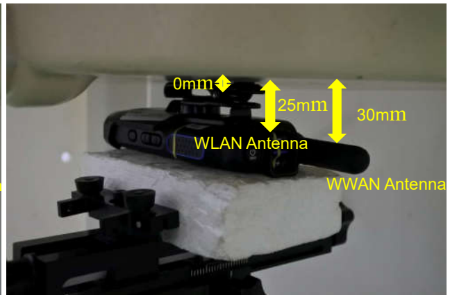
Back with Swivel Carry Holster, Test Separation 0 mm
