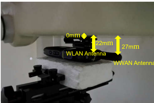
Back with Belt Clip, Test Separation 0 mm
