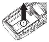
2 With the contacts facing down, align the card notched end first and slide the SIM card into the slot.
