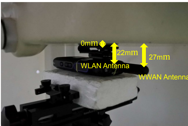
Back with Belt Clip, Test Separation 0 mm
