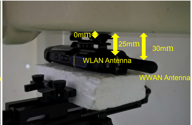
Back with Swivel Carry Holster, Test Separation 0 mm
