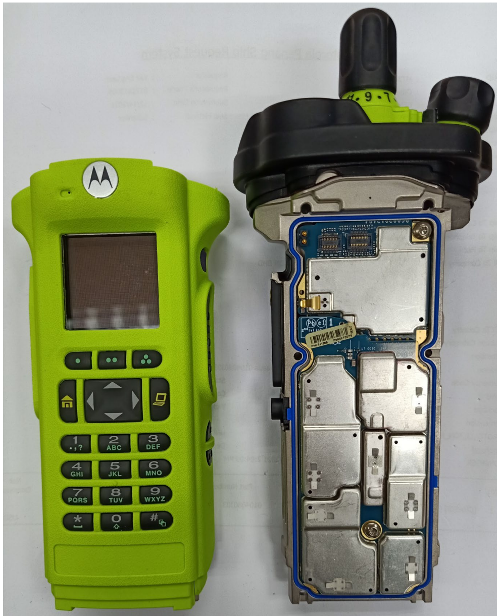
RF and Vocon boards with chassis and housing of APX8000HXE Model 3.5 (Front side)
