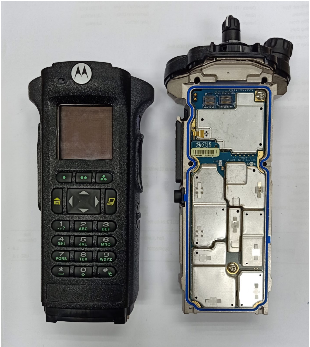
RF and Vocon boards with chassis and housing of APX8000H Model 3.5 BLK/BRN (Front side)
