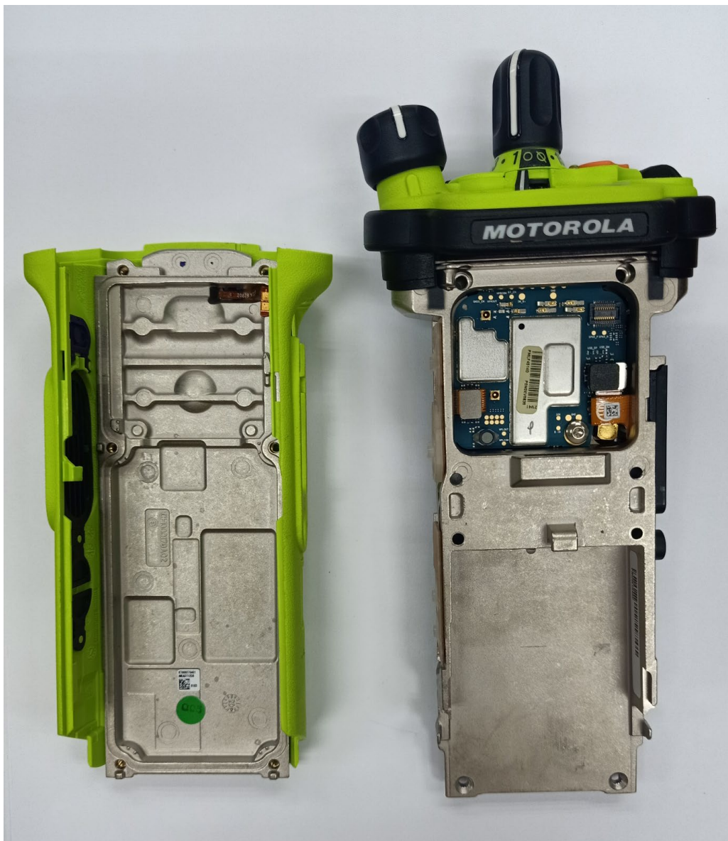
Expansion board with chassis and housing of APX8000HXE Model 1.5 (Back side)
