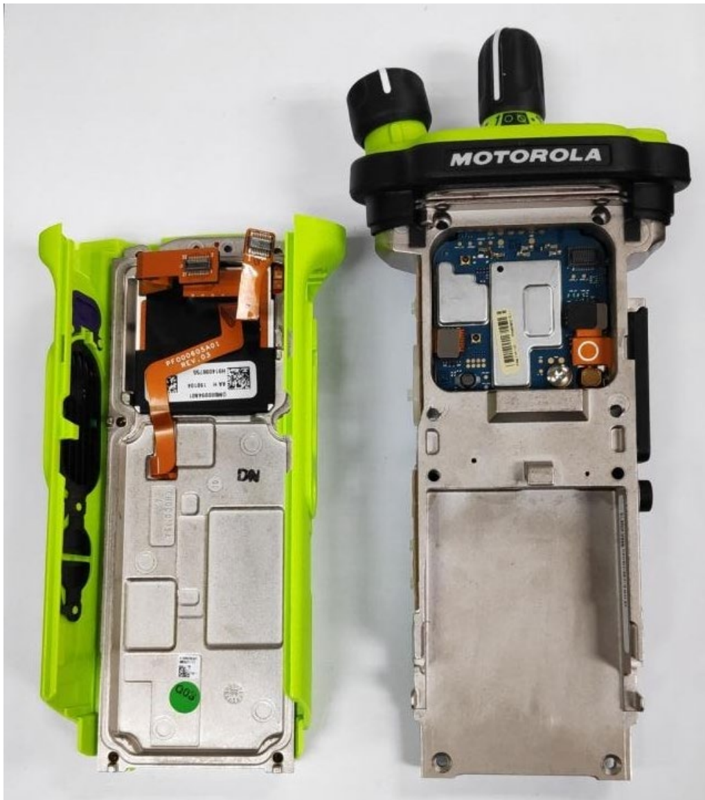
Expansion board with chassis and housing of APX8000HXE Model 2.5 (Back side)
