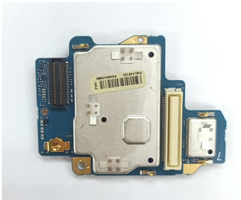
Vocon board with shields (Bottom) (APX8000H/ APX8000HXE)
