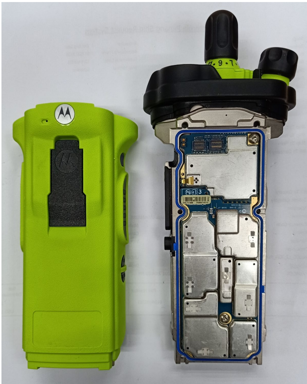
RF and Vocon boards with chassis and housing of APX8000HXE Model 1.5 (Front side)
