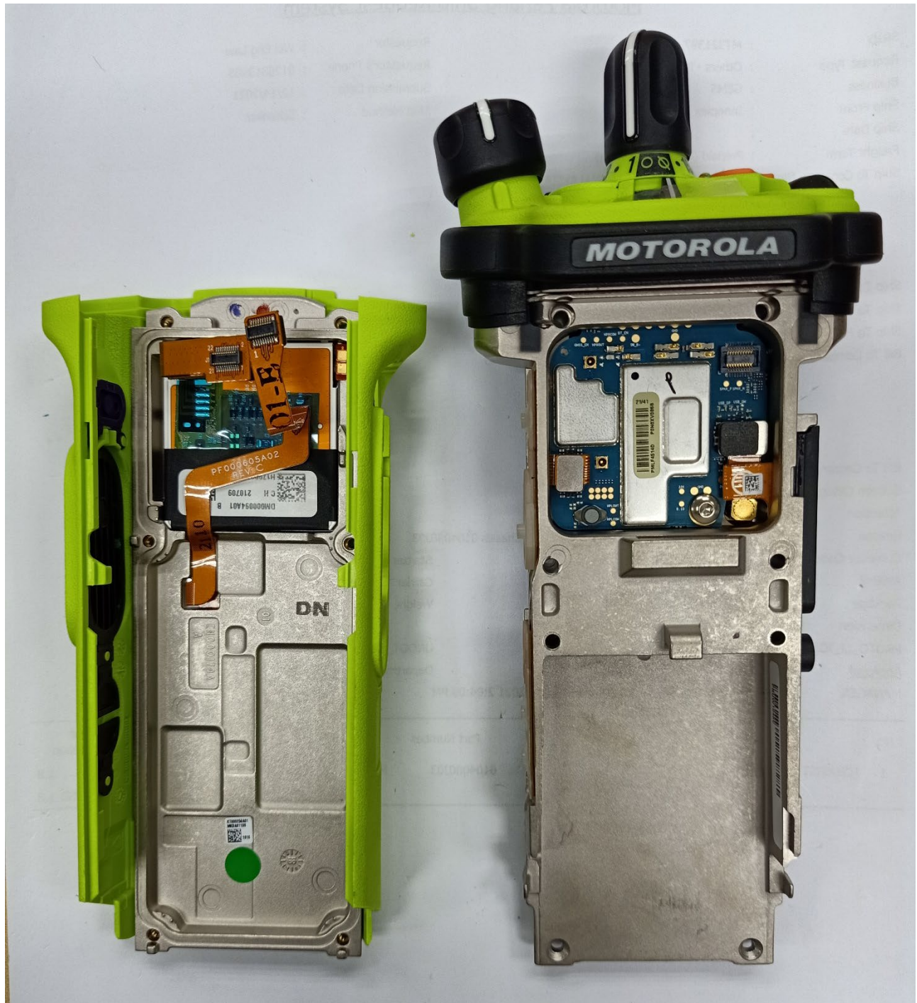
Expansion board with chassis and housing of APX8000HXE Model 3.5 (Back side)
