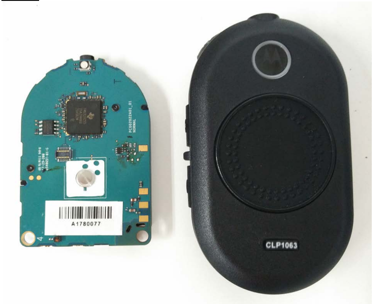
RF board with housing (front side) (Same between CLP1060, CLP1063, only front nameplate label change)
