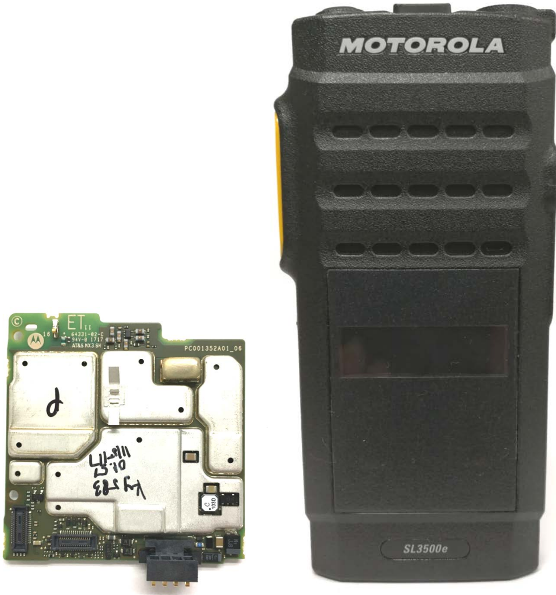
RF board with chassis and housing (front)
