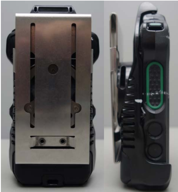
PMLN7699A Carry holster with metal pocket clip. (DUT Front Back & Side View).
