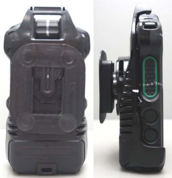
PMLN7700A Carry holster with Peter Jones mounting stud and GMDN0386A Klick fast sew on dock. (DUT Back & Side View).
