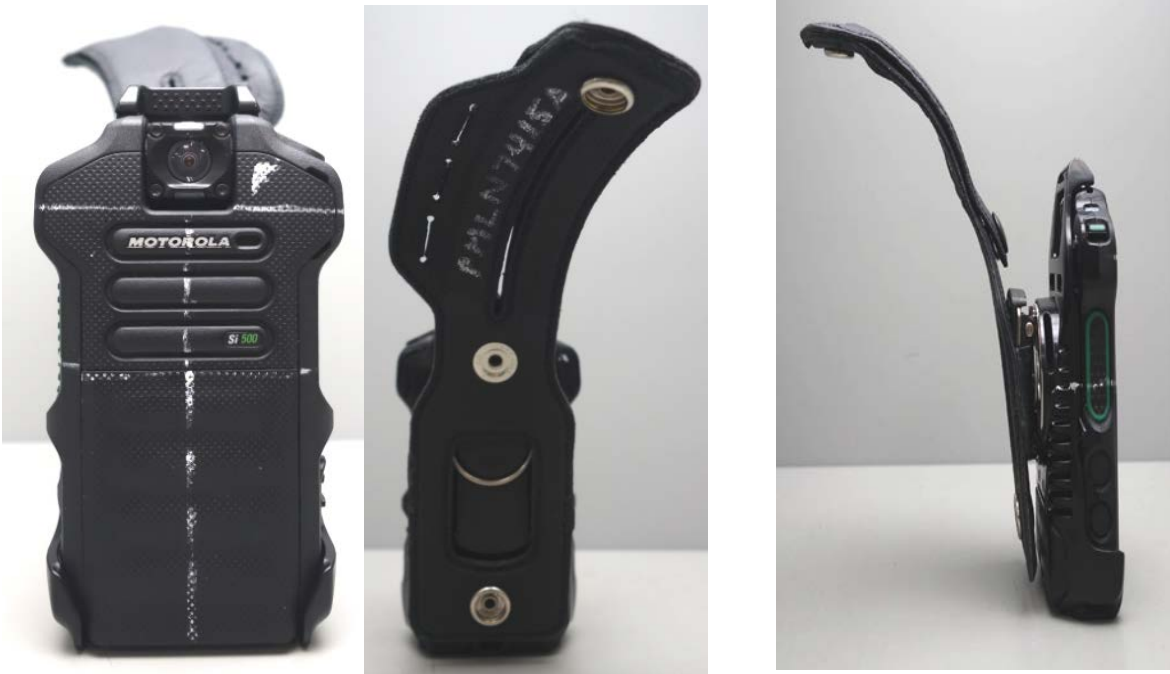
PMLN7698A carry holster with swivel clip and PMLN7415A shoulder epaulette strap. (DUT Front, Back & Side View)
