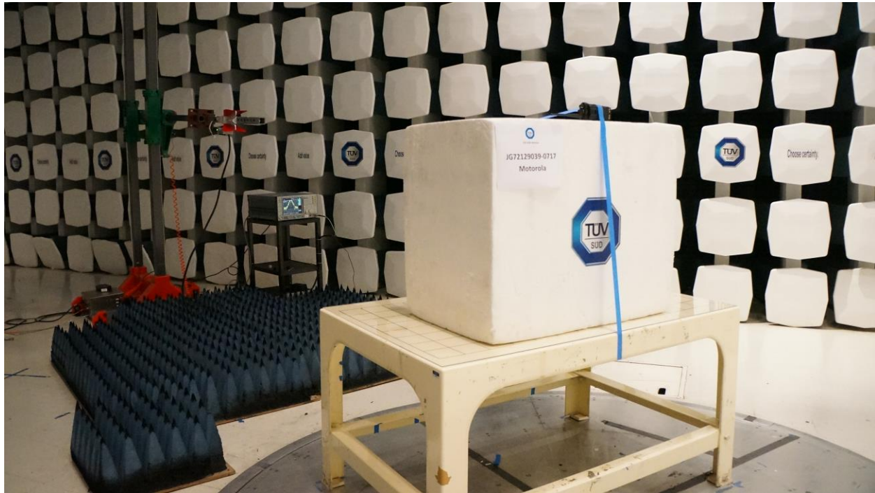
Radiated Emissions Test Setup (Above 1000 MHz - Back)
