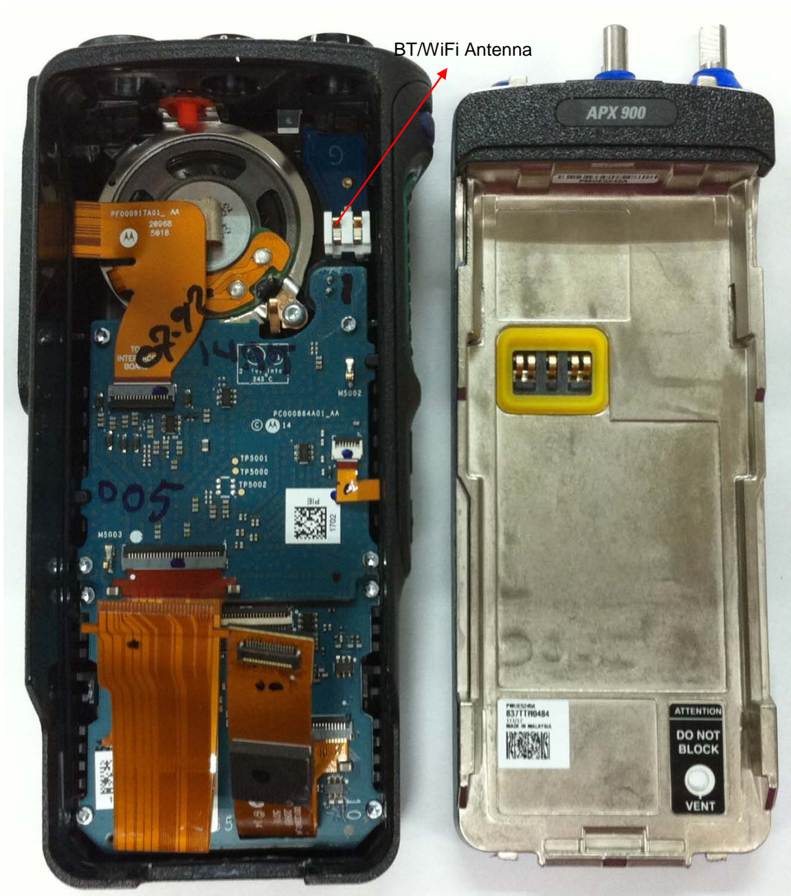
Chassis and housing (Back Side), Model 2 (APX900)
