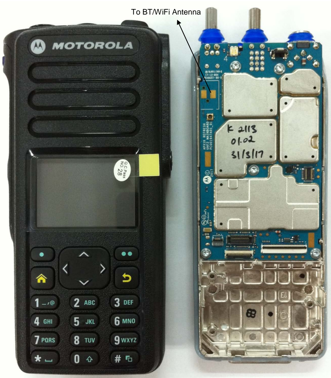
RF boards with chassis and housing (Front Side), Model 3 (APX900)
