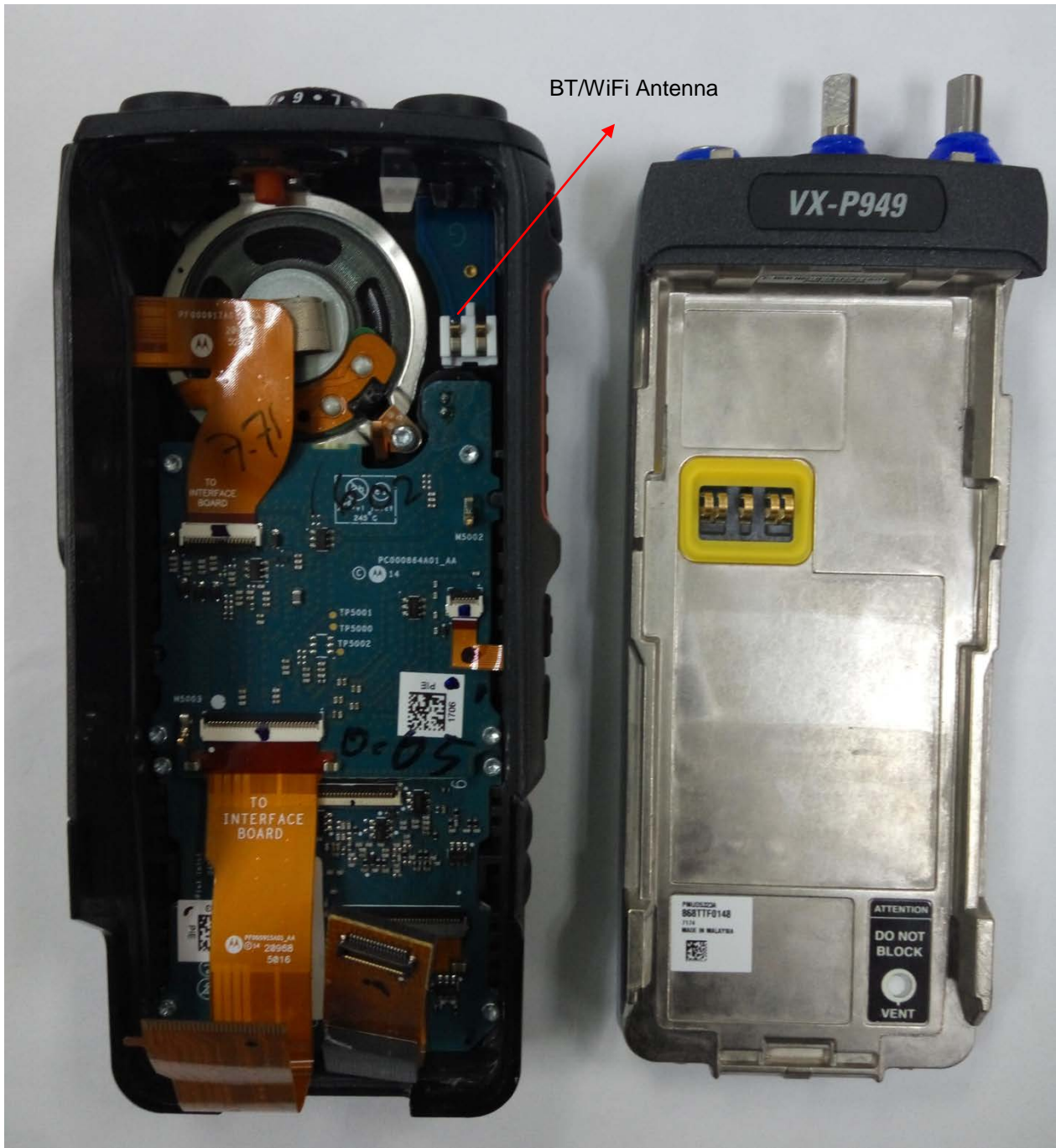
Chassis and housing for (Back Side), Model 3 (VX-P949)
