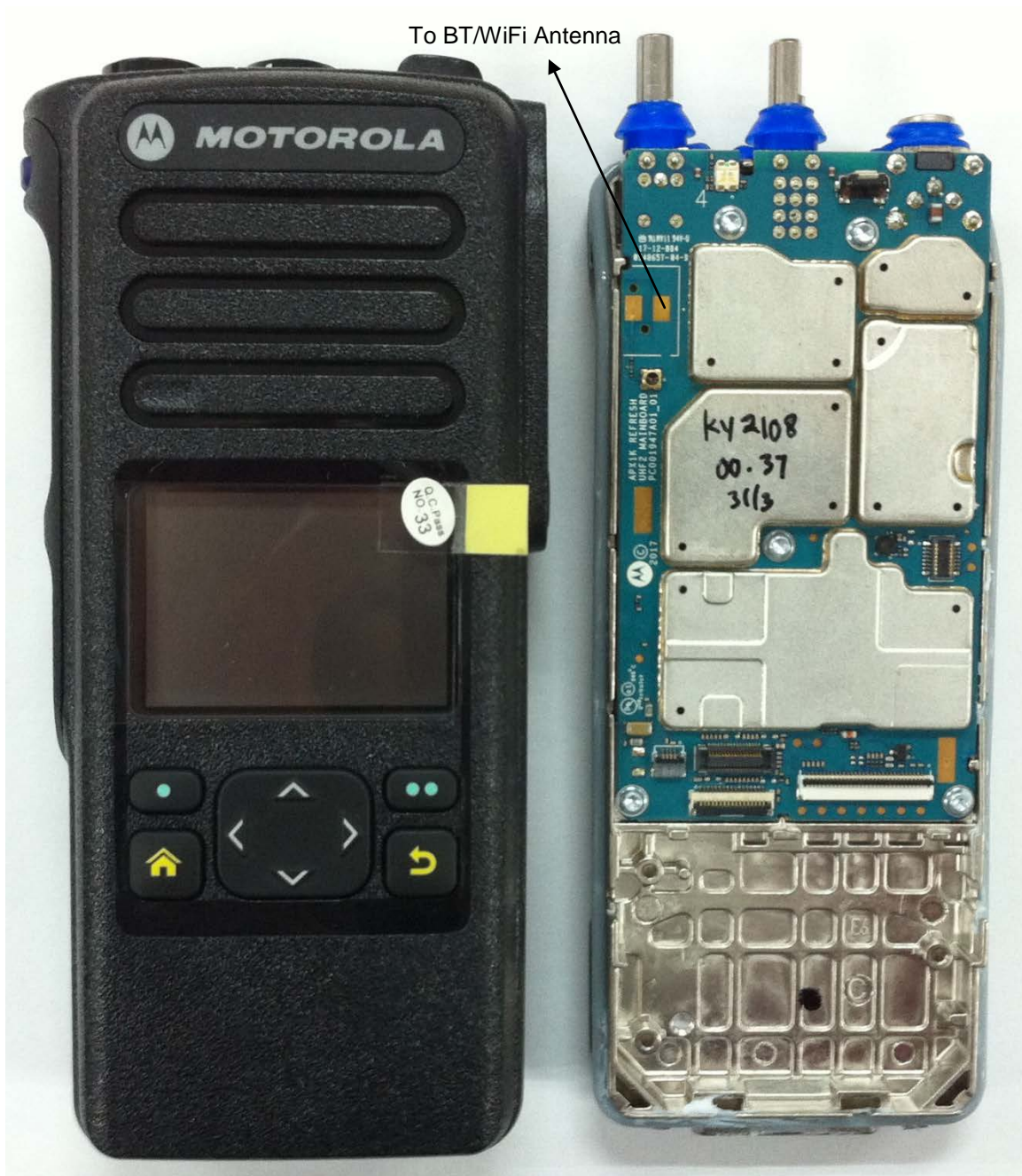
RF boards with chassis and housing (Front Side), Model 2 (APX900)
