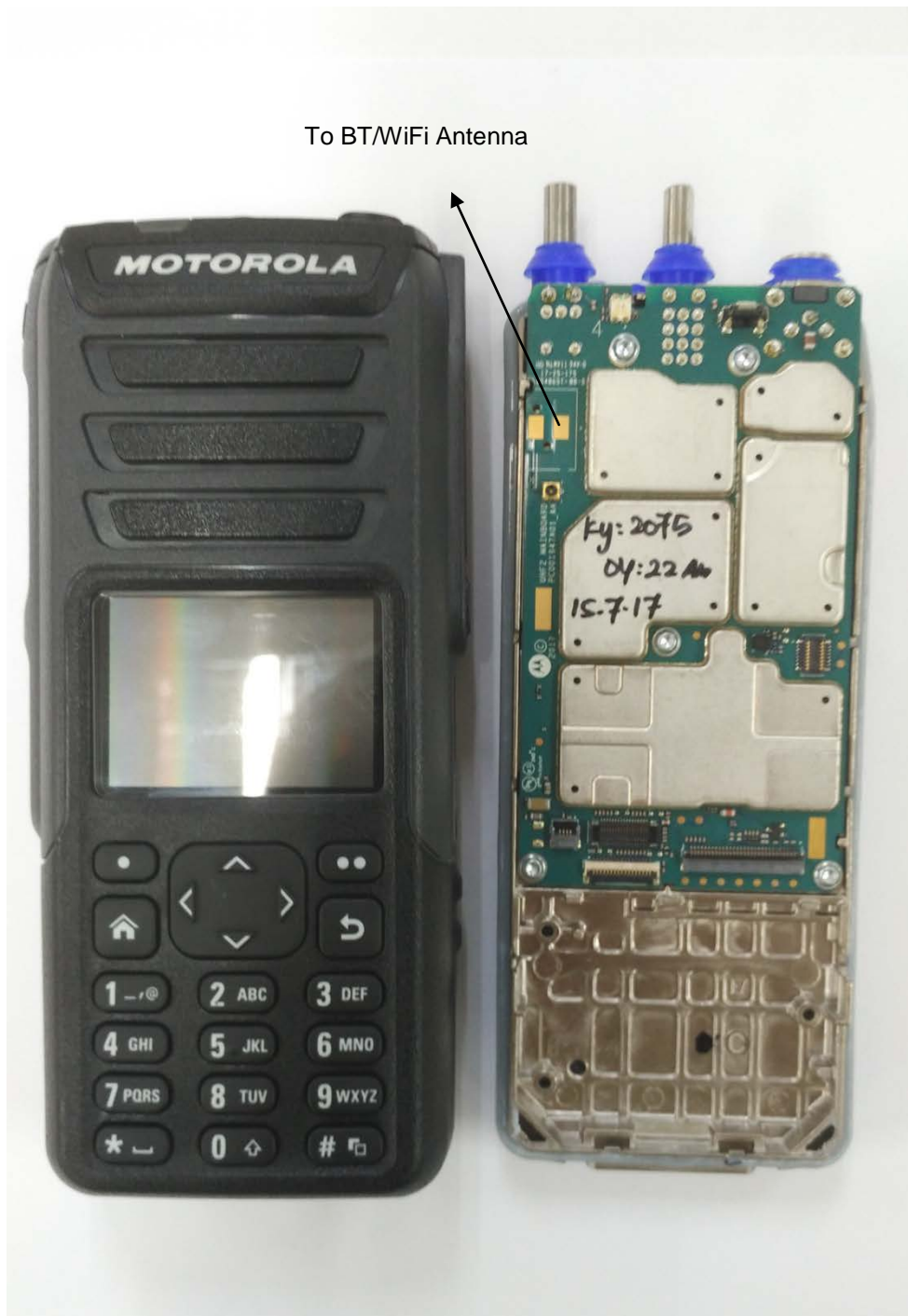
RF boards with chassis and housing (Front Side), Model 3 (VX-P949)
