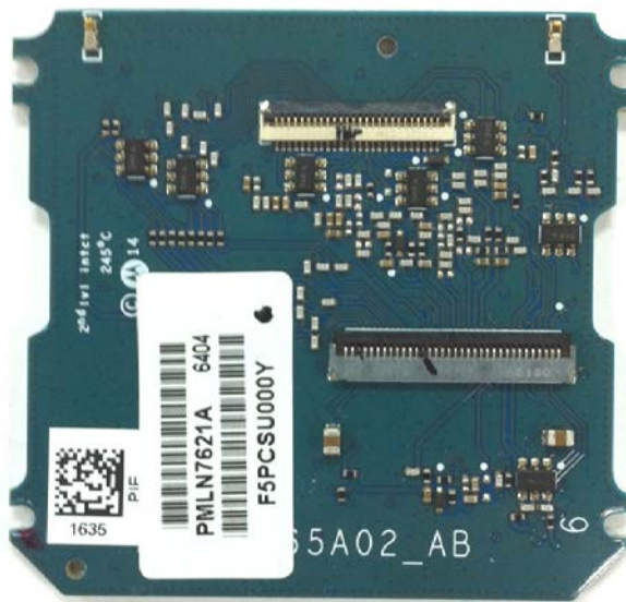
Keypad Board (Bottom), Model 3 (APX900 & VX-P949)
