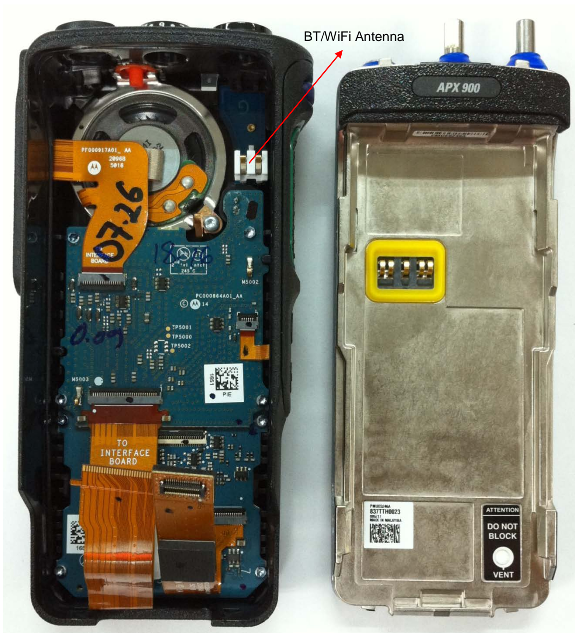
Chassis and housing for (Back Side), Model 3 (APX900)
