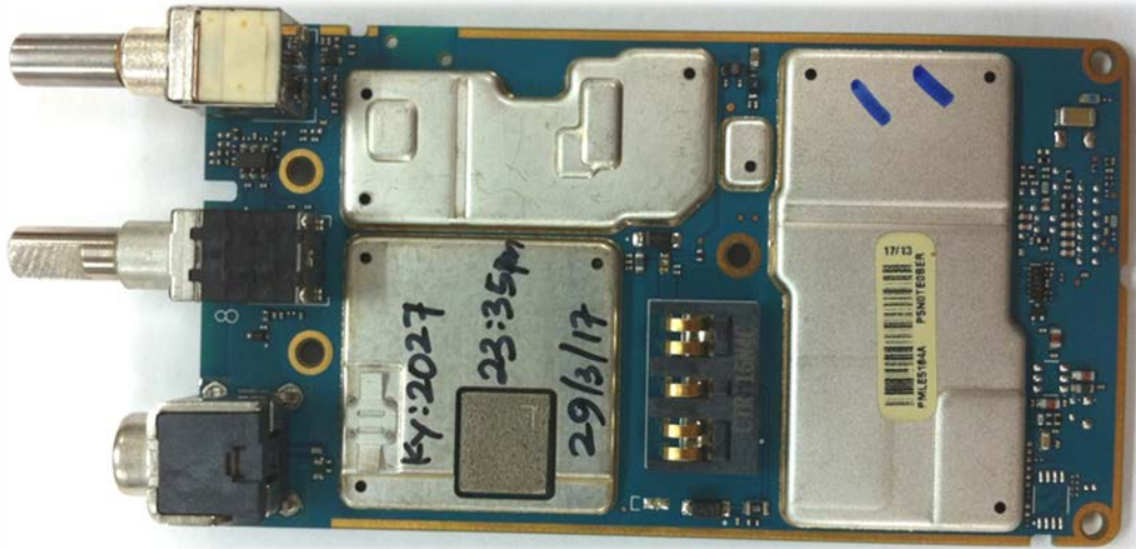
RF board with Shields (Bottom) (APX900 & VX-P949)
