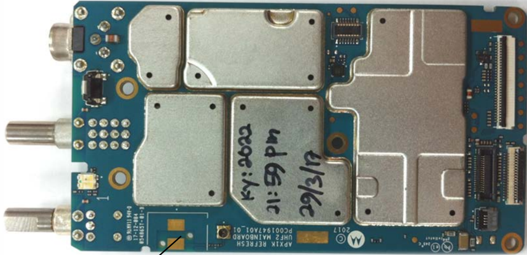
RF board with Shields (Top) (APX900 & VX-P949)
