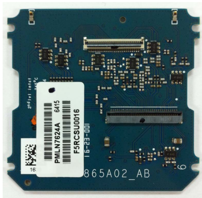
Keypad Board (Bottom), Model 2 (APX900)
