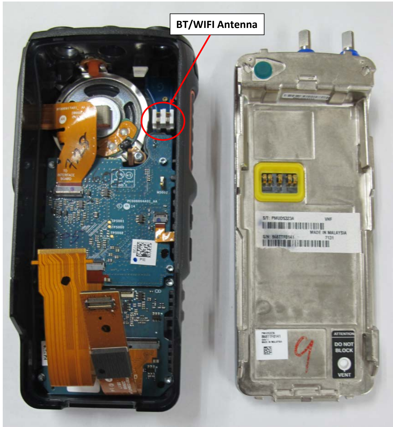
Chassis and Housing (Back), Model 3 (VX-P949)
