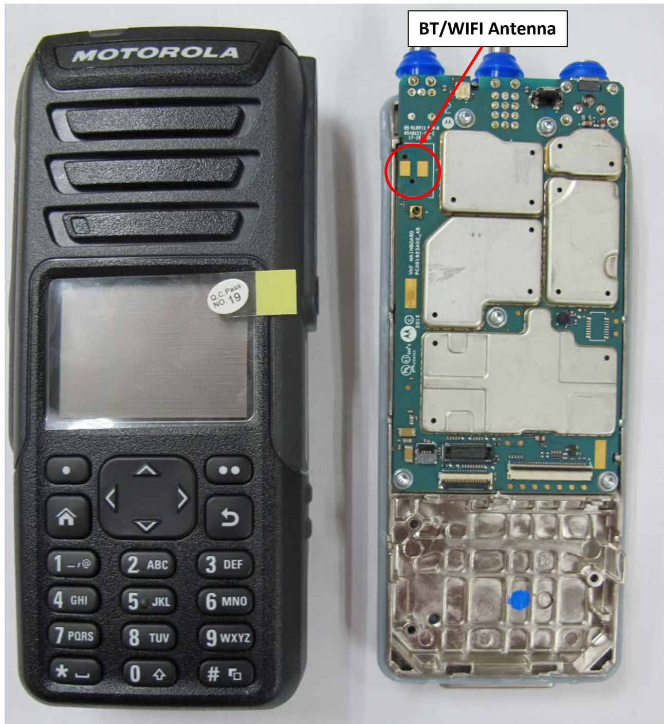
RF board with chassis and housing (front) Model 3 (VX-P949)
