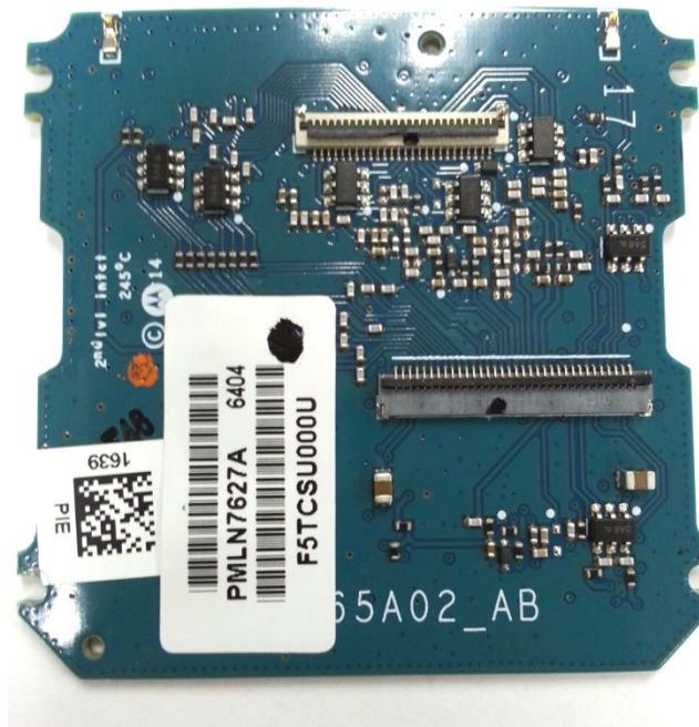
Keypad board (Bottom), Model 2 (APX900)
