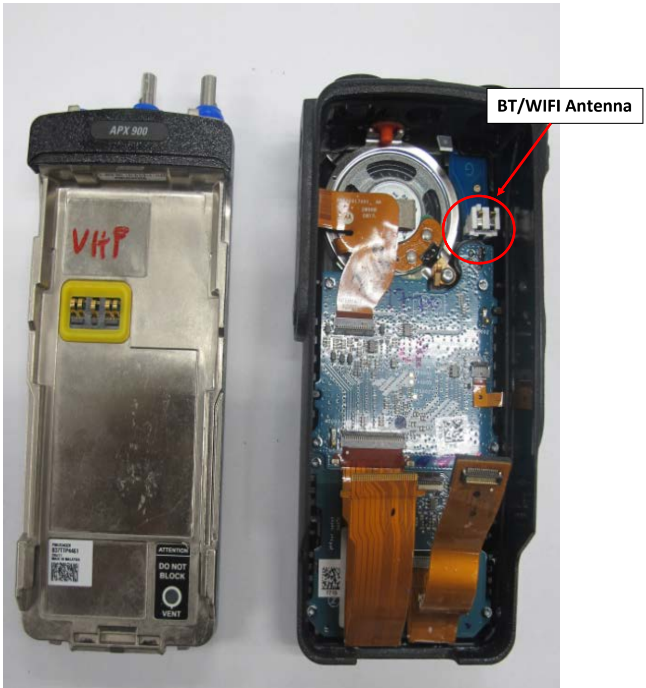
Chassis and Housing (Back), Model 3 (APX900)
