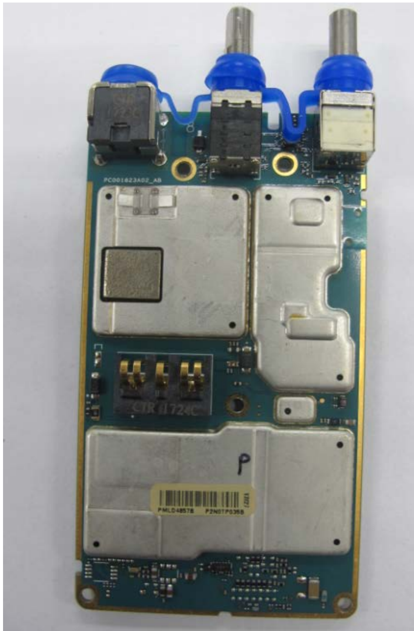
RF board with Shields (Bottom) (APX900 & VX-P949)
