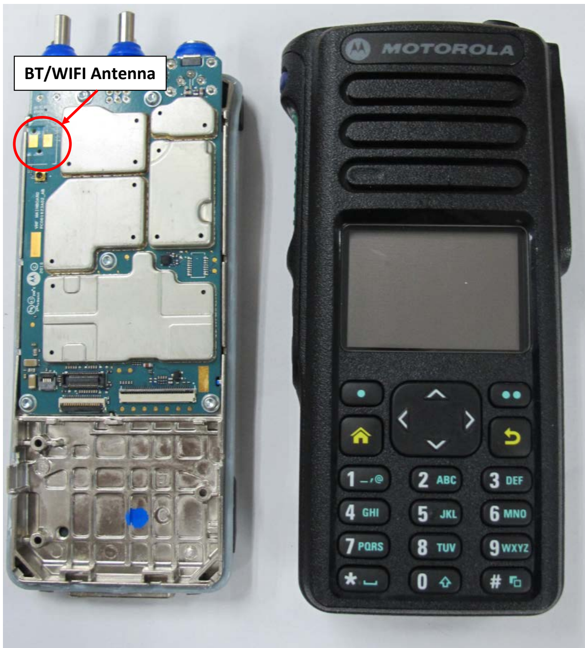
RF board with chassis and housing (front) Model 3 (APX900)
