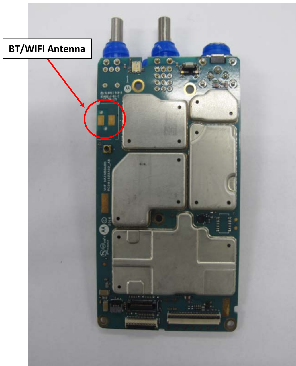
RF board with Shields (Top) (APX900 & VX-P949)
