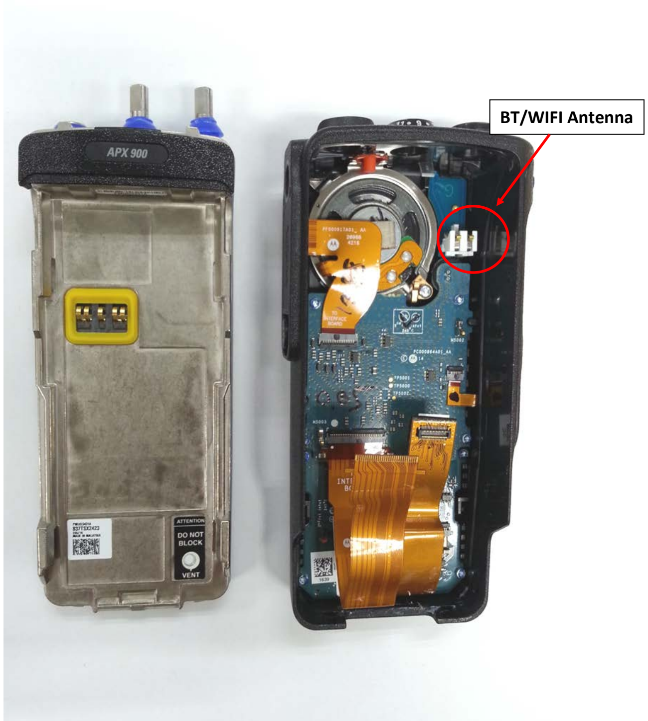
Chassis and Housing (Back), Model 2 (APX900)
