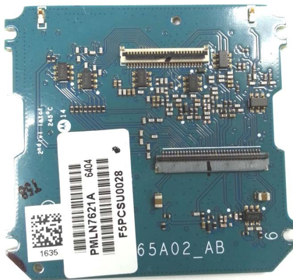
Keypad board (Bottom), Model 3 (VX-P949)
