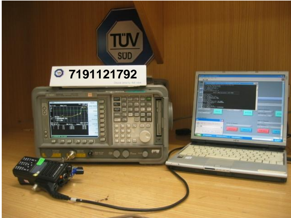
Spectrum Bandwidth (6dB Bandwidth Measurement) Test Setup
