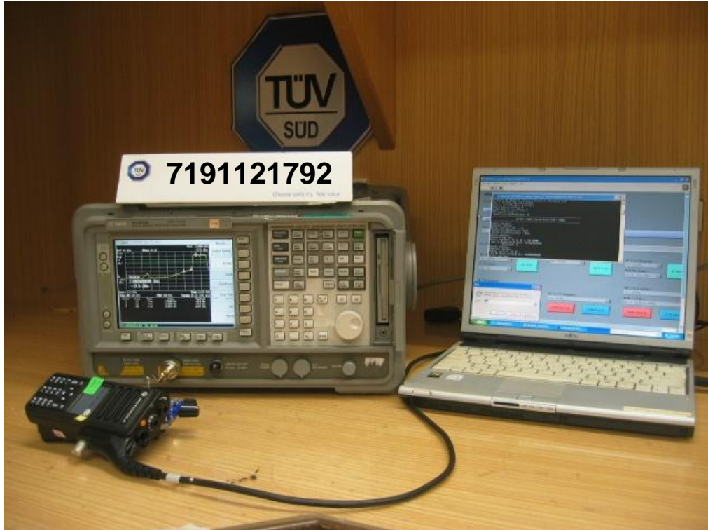
RF Conducted Spurious Emissions (Non-Restricted Bands) Test Setup
