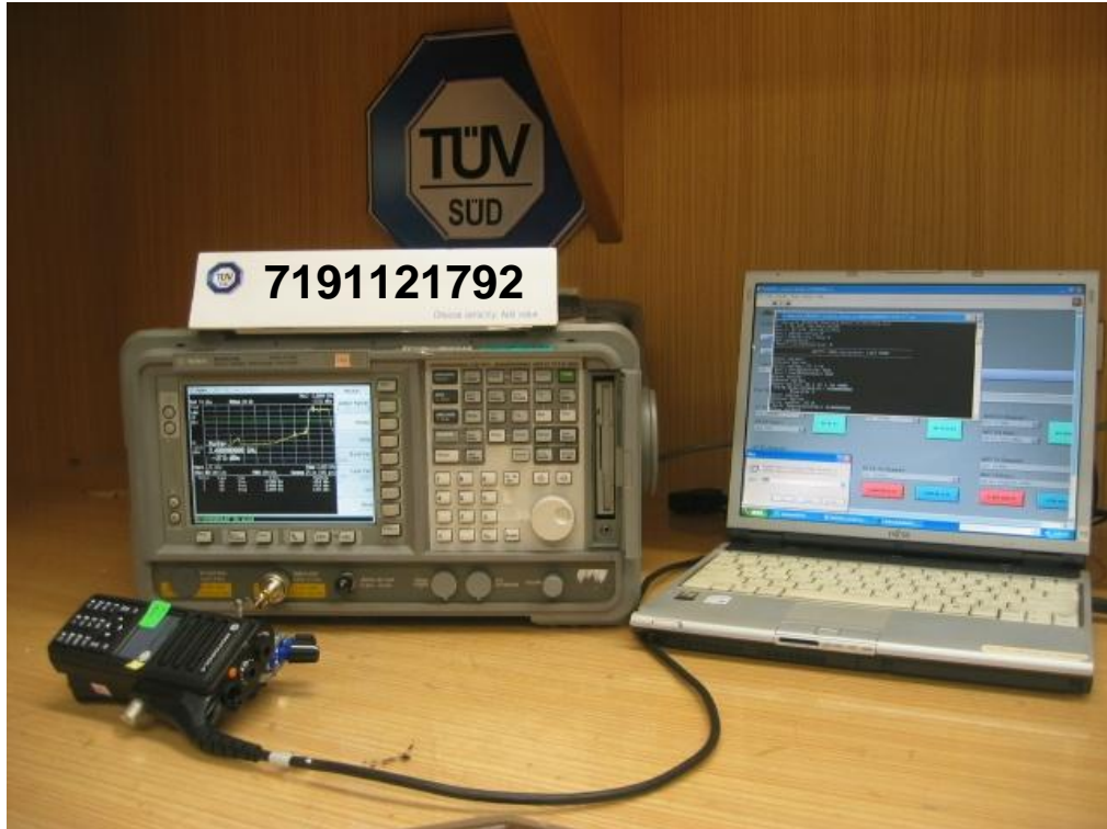
Peak Power Spectral Density Test Setup
