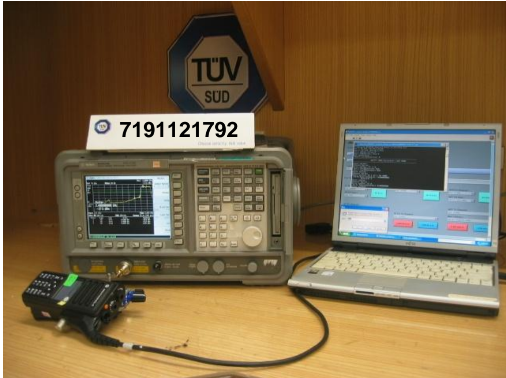
Band Edge Compliance (Conducted) Test Setup
