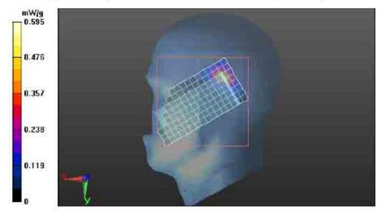
Shortened scan reflect highest SAR producing configuration; approximate run time is 21 minutes. Representative full scan run time was 35 minutes.
