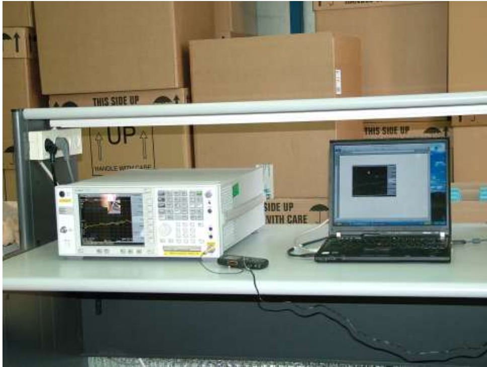
Photograph 1: Conducted measurements at the antenna port
