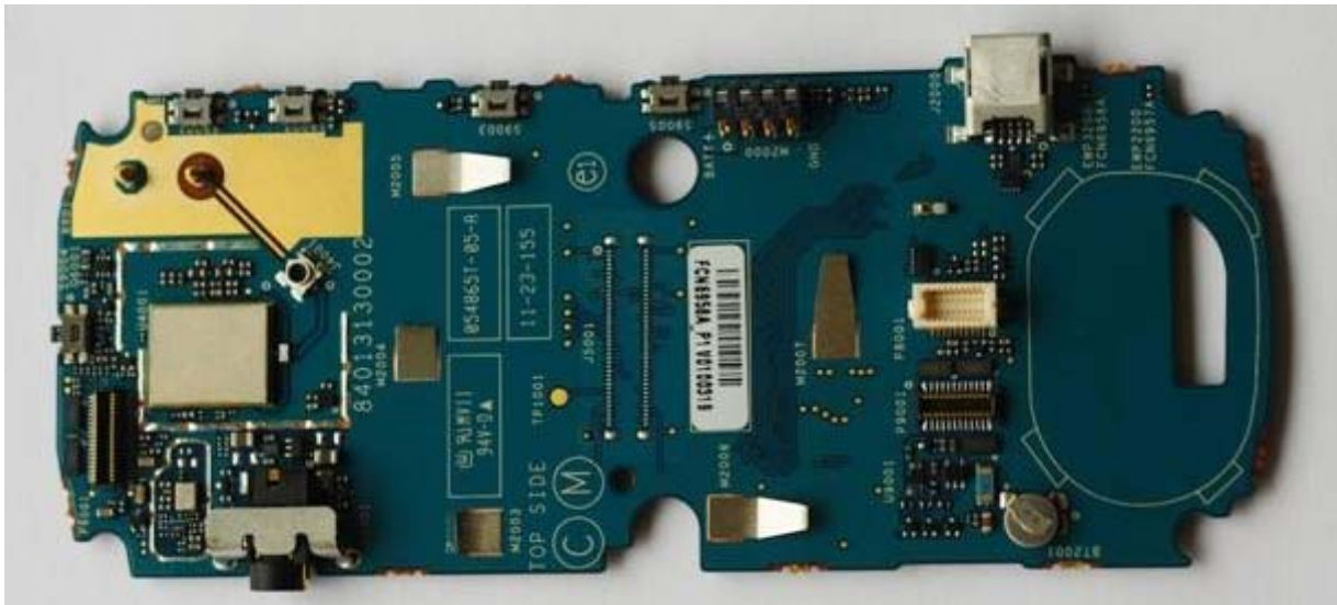
Photograph 3 – EWP3200 Rear PCB Top View Shields Removed
