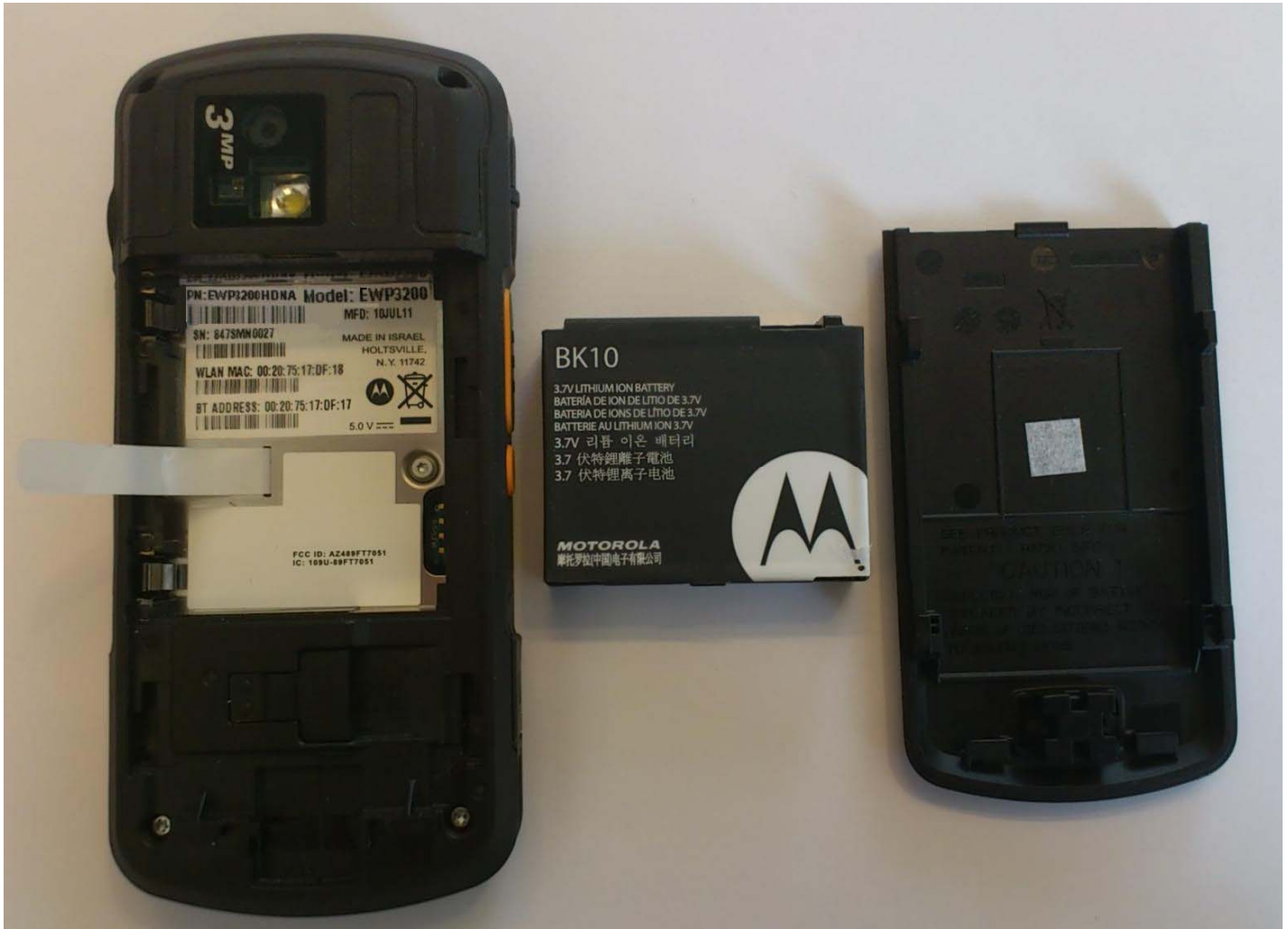
Photograph 5 – EWP3200 Assembly of Battery and Battery Cover
