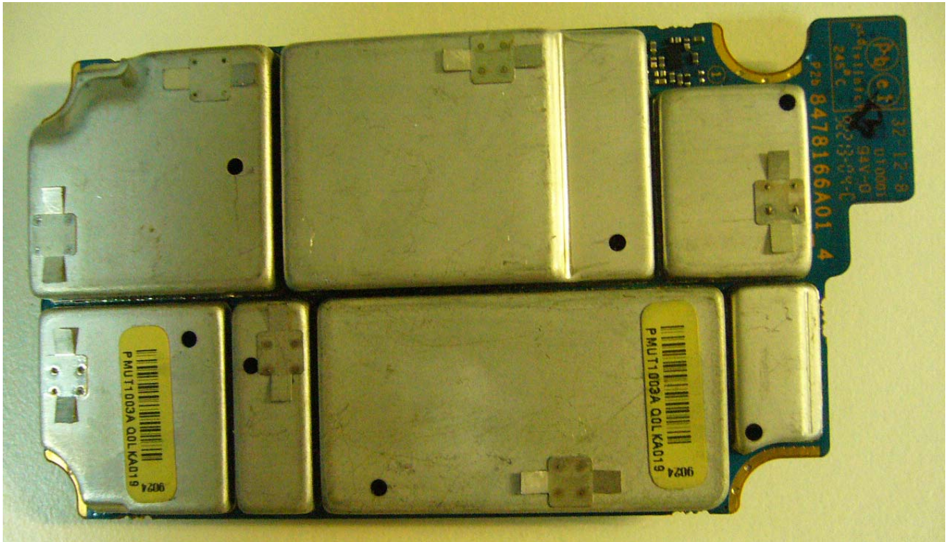
RF board with Shields (Bottom)
