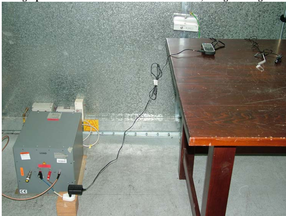
Photograph 2: Power Line Emissions measurement, charger configuration
