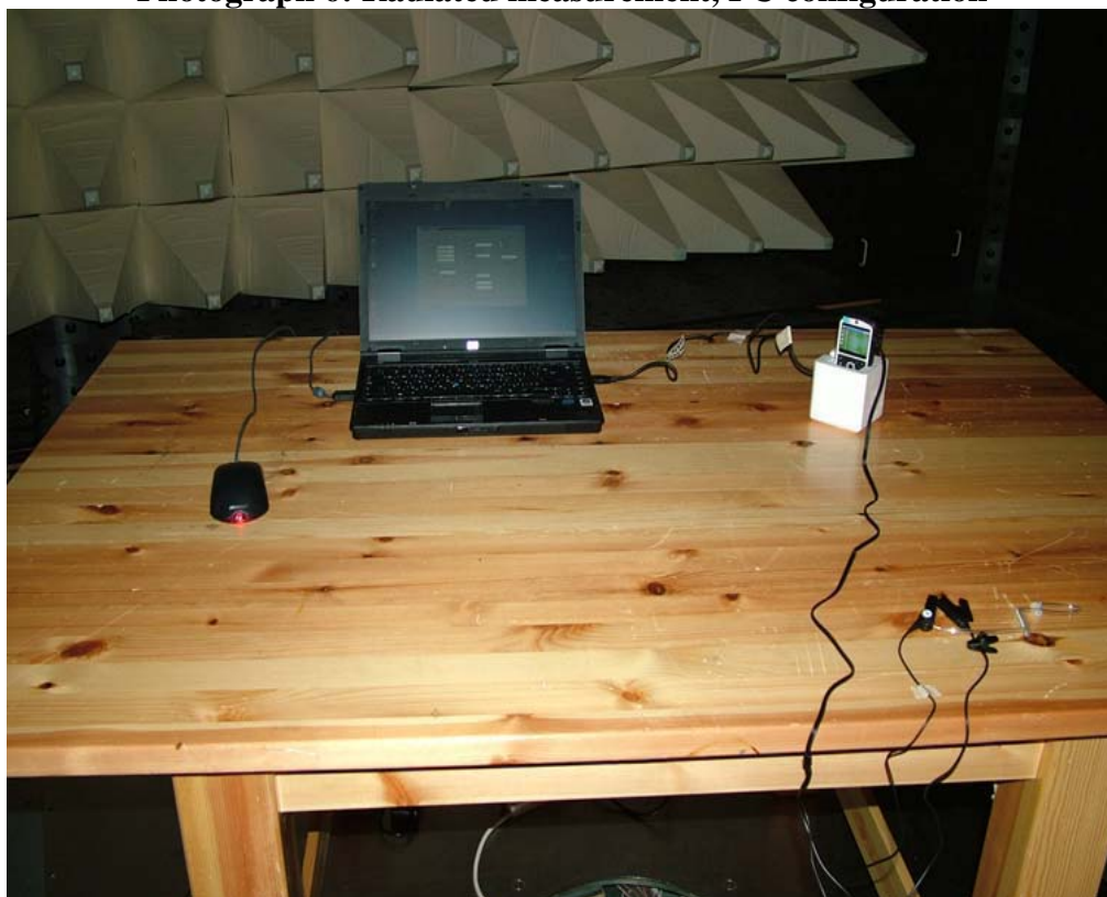
Photograph 6: Radiated measurement, PC configuration
