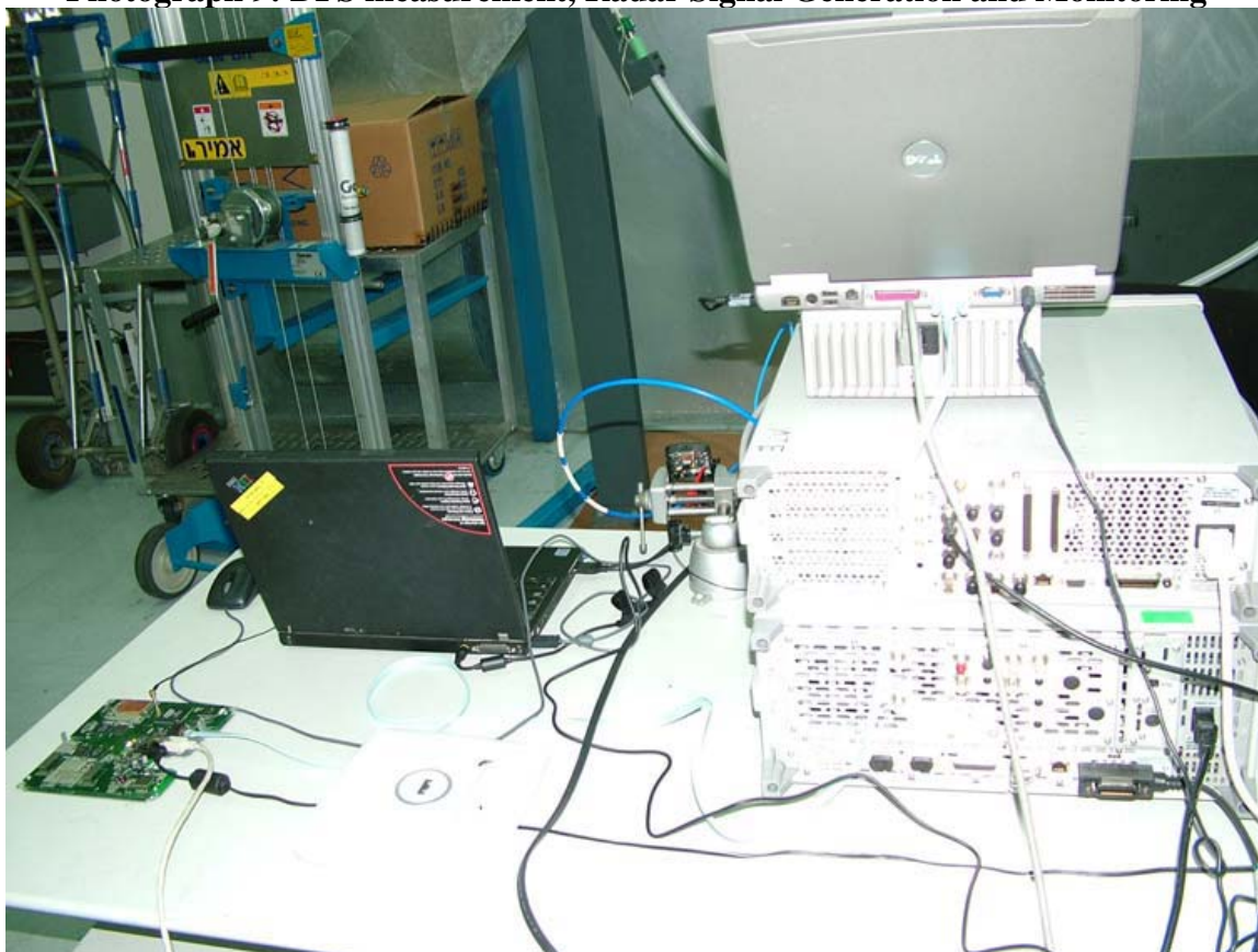
Photograph 9: DFS measurement, Radar Signal Generation and Monitoring
