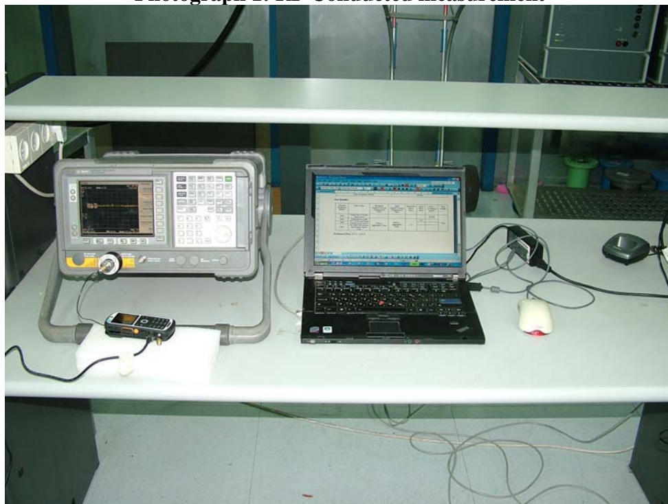
Photograph 1: RF Conducted measurement
