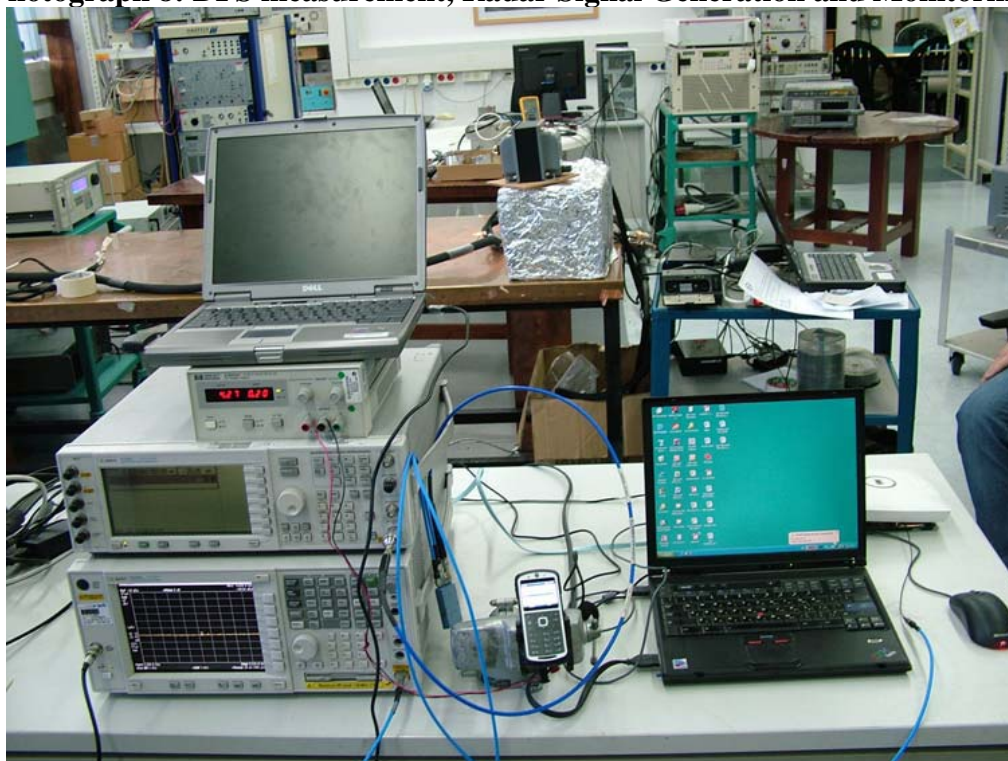
Photograph 8: DFS measurement, Radar Signal Generation and Monitoring,
