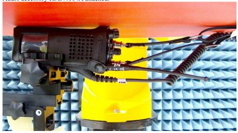
DUT with accessory side against the phantom with carry accessory PMLN5328A and NTN5243A. Audio accessory HMN4104A attached.
