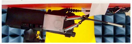
DUT with back side against the phantom with carry accessory PMLN5330A and NTN5243A. Audio accessory HMN4104A attached.
