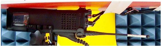
DUT with accessory side against the phantom with carry accessory PMLN5330A and NTN5243A. Audio accessory HMN4104A attached.
