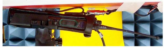
DUT with PTT side against the phantom with carry accessory PMLN5329A and NTN5243A. Audio accessory HMN4104A attached.
