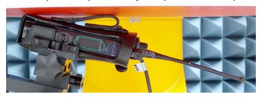
DUT with carry accessory PMLN5324A/PMLN5407A 2.5" swivel loop against the phantom. Audio accessory HMN4104A attached.
