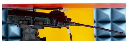
DUT with accessory side against the phantom with carry accessory PMLN5322A and NTN5243A. Audio accessory HMN4104A attached.
