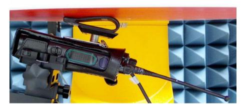
DUT with carry accessory PMLN5324A/PMLN5408A 2.75" swivel loop against the phantom. Audio accessory HMN4104A attached.
