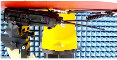
DUT with PTT side against the phantom with carry accessory PMLN5322A and NTN5243A. Audio accessory HMN4104A attached.
