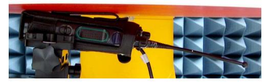
DUT with carry case accessory PMLN5323A against the phantom. Audio accessory HMN4104A attached.
