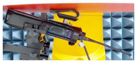
DUT with carry accessory PMLN5330A/PMLN5408A 2.75" swivel loop against the phantom. Audio accessory HMN4104A attached.
