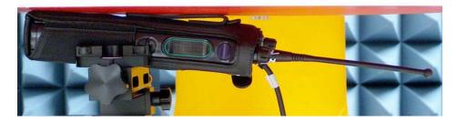
DUT with carry accessory PMLN5329A against the phantom. Audio accessory HMN4104A attached.
