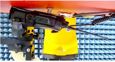
DUT with PTT side against the phantom with carry accessory PMLN5324A and NTN5243A. Audio accessory HMN4104A attached.
