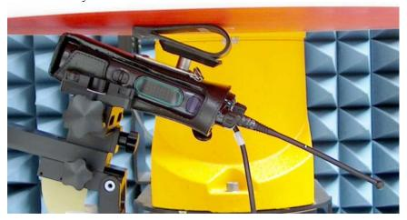
DUT with carry accessory PMLN5324A/PMLN5409A 3.0" swivel loop against the phantom. Audio accessory HMN4104A attached.
