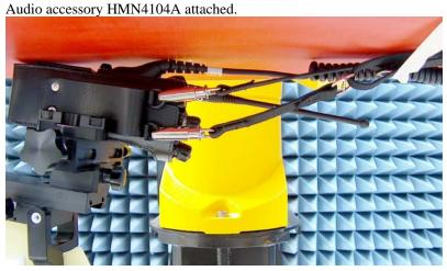
DUT with back side against the phantom with carry accessory PMLN5323A and NTN5243A. Audio accessory HMN4104A attached.
