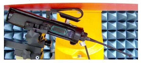
DUT with carry accessory PMLN5330A/PMLN5409A 3.0" swivel loop against the phantom. Audio accessory HMN4104A attached.
