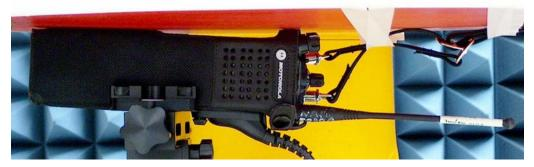
DUT with accessory side against the phantom with carry accessory PMLN5329A and NTN5243A. Audio accessory HMN4104A attached.
