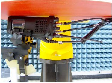
DUT with accessory side against the phantom with carry accessory PMLN5324A and NTN5243A. Audio accessory HMN4104A attached.
