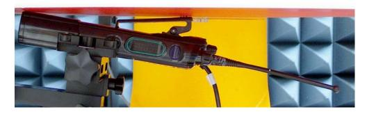
DUT with belt clip NTN8266B against the phantom. Audio accessory HMN4104A attached. (Same position used for all other tested audio accessories)
