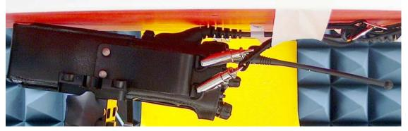
DUT with back side against the phantom with carry accessory PMLN5329A and NTN5243A. Audio accessory HMN4104A attached.
