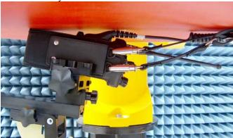
DUT with back side against the phantom with carry accessory PMLN5322A and NTN5243A. Audio accessory HMN4104A attached.
