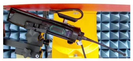
DUT with carry accessory PMLN5328A against the phantom. Audio accessory HMN4104A attached.
