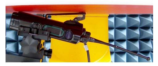
DUT with carry accessory PMLN5331A and belt clip NTN8266B against the phantom. Audio accessory HMN4104A attached.
