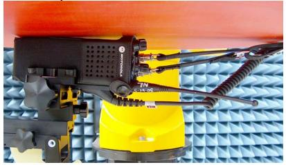
DUT with accessory side against the phantom with carry accessory PMLN5323A and NTN5243A.
