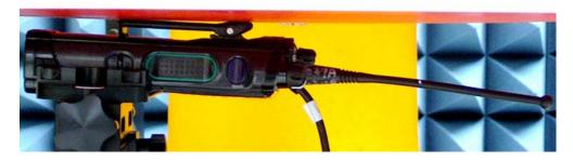
DUT with carry accessory PMLN5322A against the phantom. Audio accessory HMN4104A attached.
