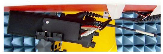
DUT with back side against the phantom with carry accessory PMLN5328A and NTN5243A. Audio accessory HMN4104A attached.
