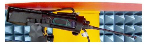
DUT with carry accessory PMLN5331A and belt clip HLN6875A against the phantom. Audio accessory HMN4104A attached.
