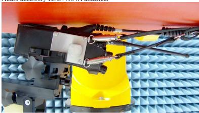
DUT with back side against the phantom with carry accessory PMLN5324A and NTN5243A. Audio accessory HMN4104A attached.
