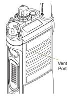
(For APX 7000 R Radios Only) The APX 7000 R radio is designed to be submerged to a maximum depth of 6 feet, with a maximum submersion time of 2 hours. Exceeding either maximum limit may result in damage to the radio.
