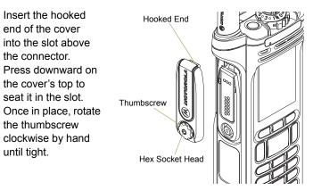
To remove the accessory connector cover, rotate the thumbscrew counterclockwise until it disengages from the radio. If the thumbscrew is too tight, use an Allen wrench to loosen it first.
