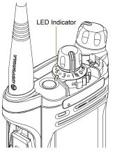
The LED lights up solid red while the radio is transmitting, and solid yellow when the radio is receiving a transmission (conventional mode only). There is no LED indication when the radio receives a transmission in trunking mode.
