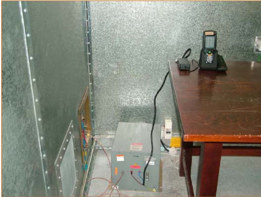
Photograph 6: HC700-L Terminal docking into Cradle configuration Conducted emission testing
