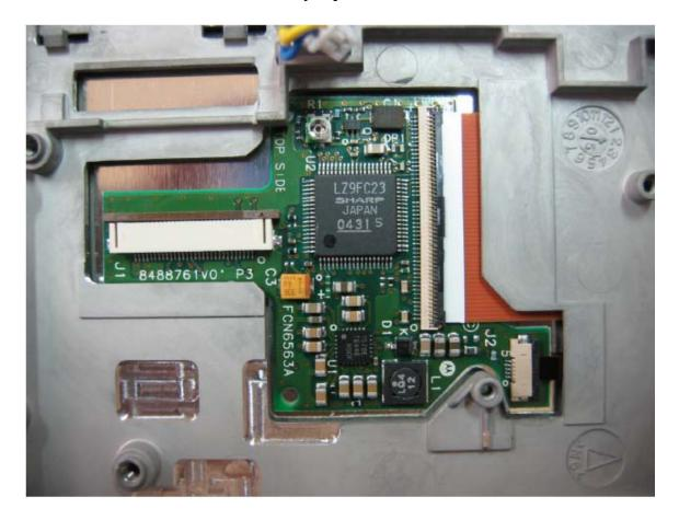
Photograph No.5 HC700-L main PCB bottom side view
