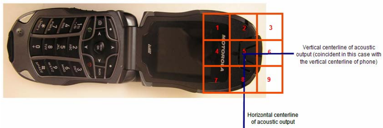
Figure A4-4. Phone Open – 5cm x 5cm grid for Near Field Measurements
