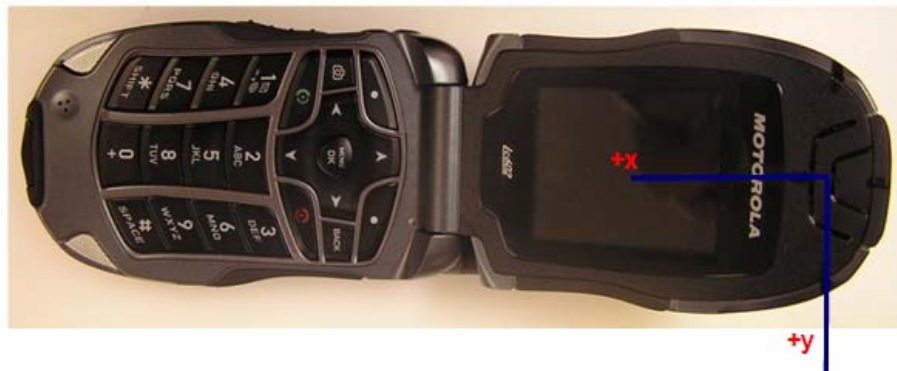
Figure A4-2. Phone Open – Coordinate Axis for T-coil Measurements
