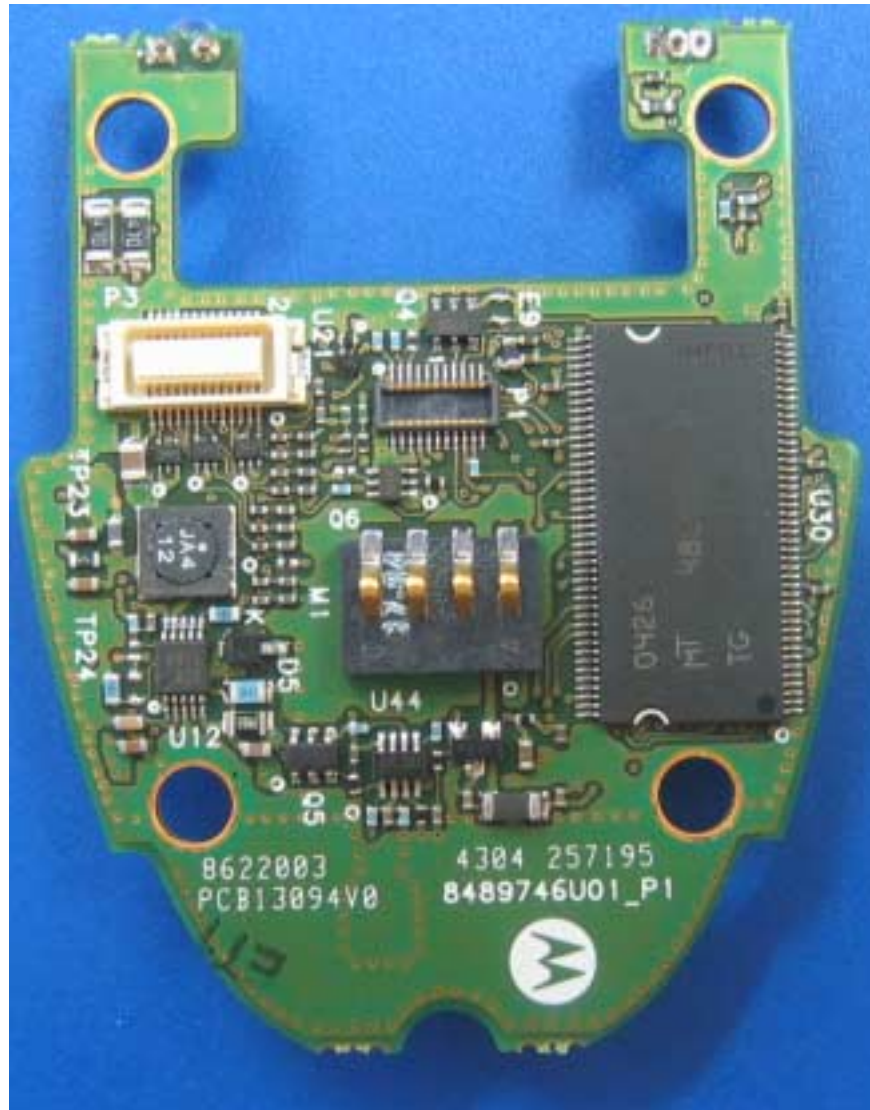
Photograph No.3 Hands Free Imager, component side of the first layer RF PCB
