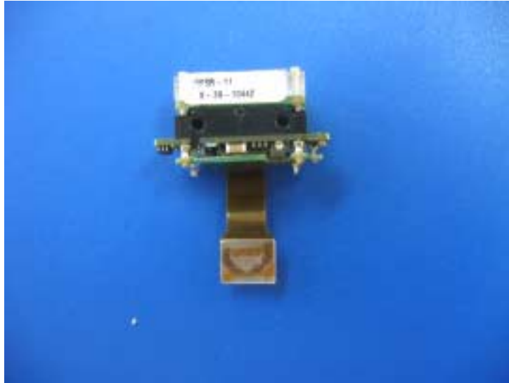
Photograph No.8 Top side of the Camera PCB
