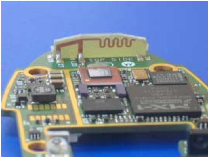
Photograph No.12 Antenna assembly view
