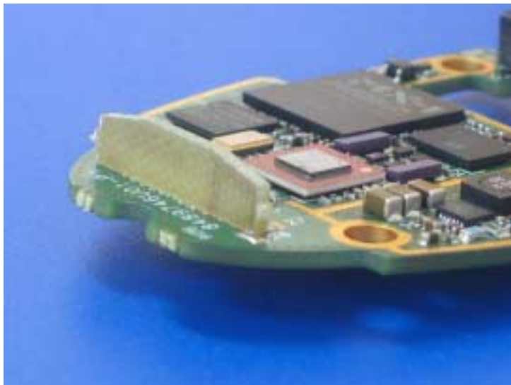
Photograph No.13 Antenna assembly view
