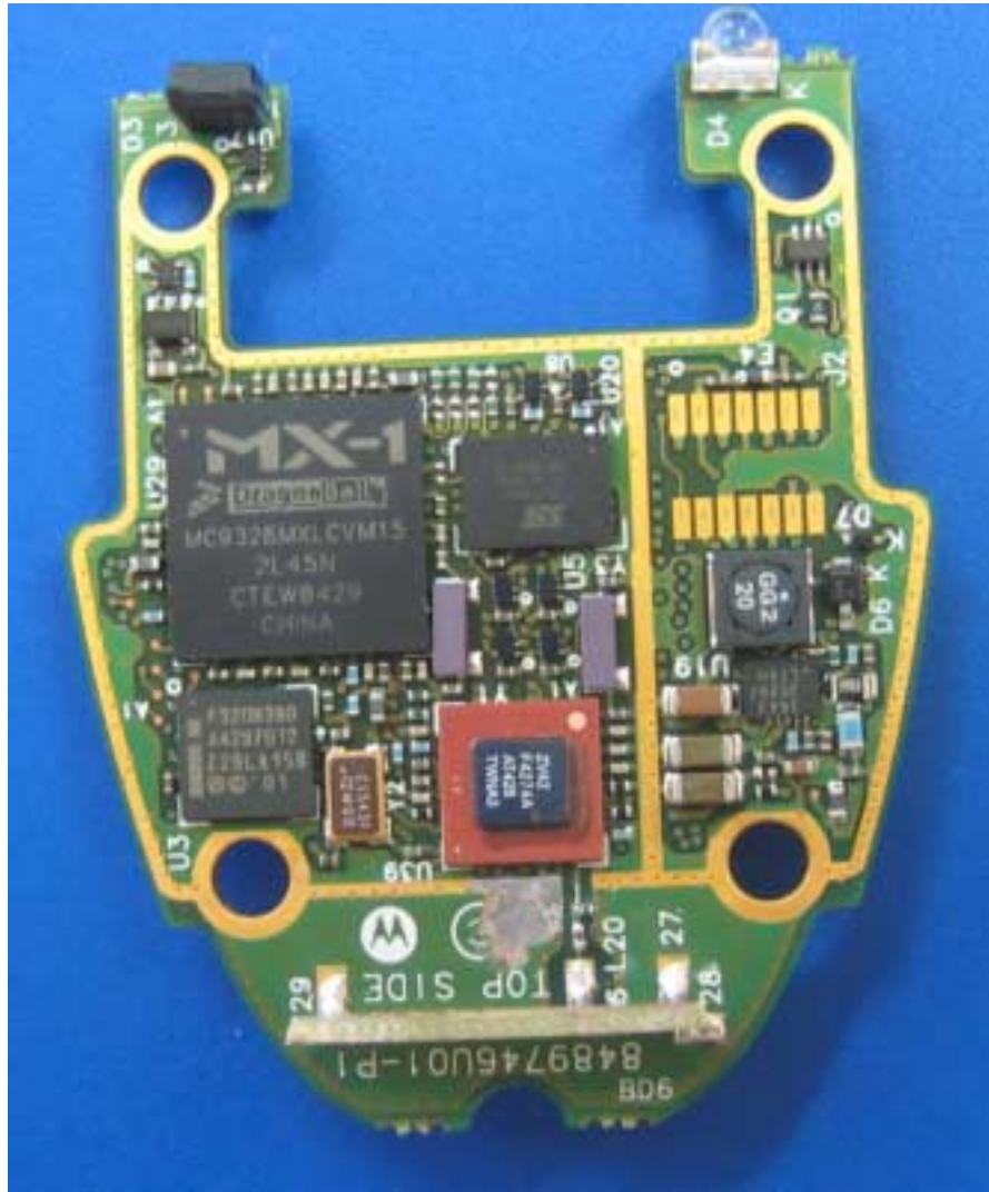
Photograph No.4 Hands Free Imager, second side of the first layer RF PCB
