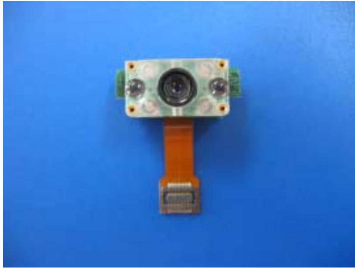
Photograph No.10 Front side of the Camera PCB
