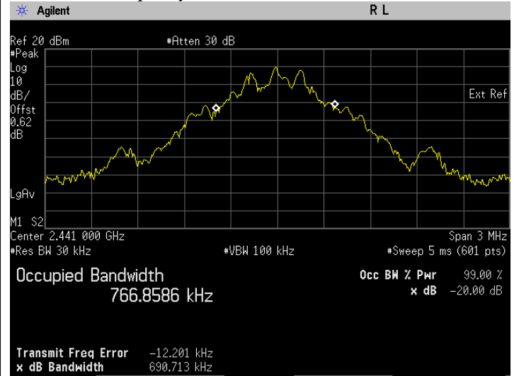
ii. The 20 dB BW & occupied bandwidth test with result at mid frequency, 8DPSK.
