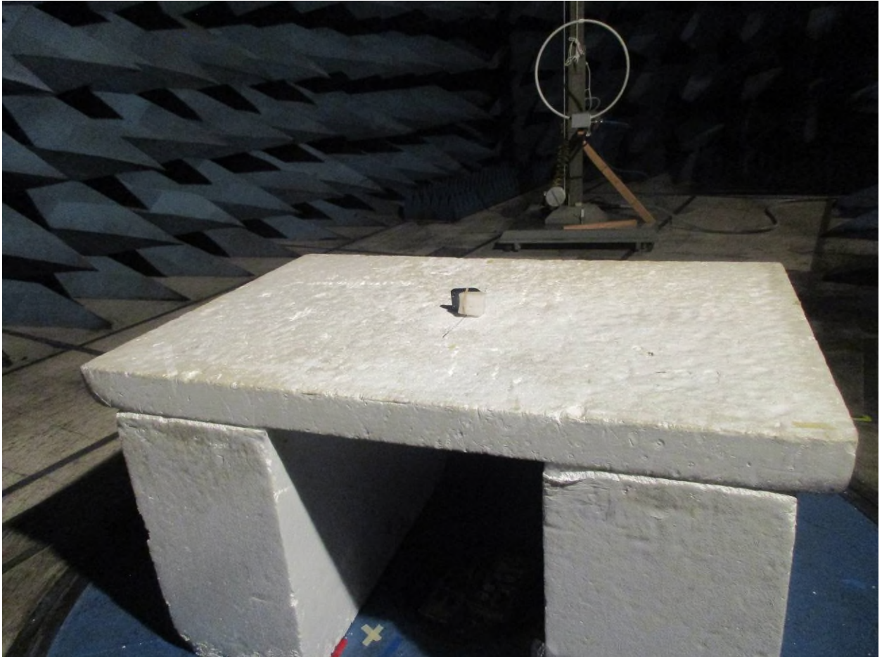
Figure 10: Radiated Emissions – Back View – EUT Sideways (below 30 MHz)
