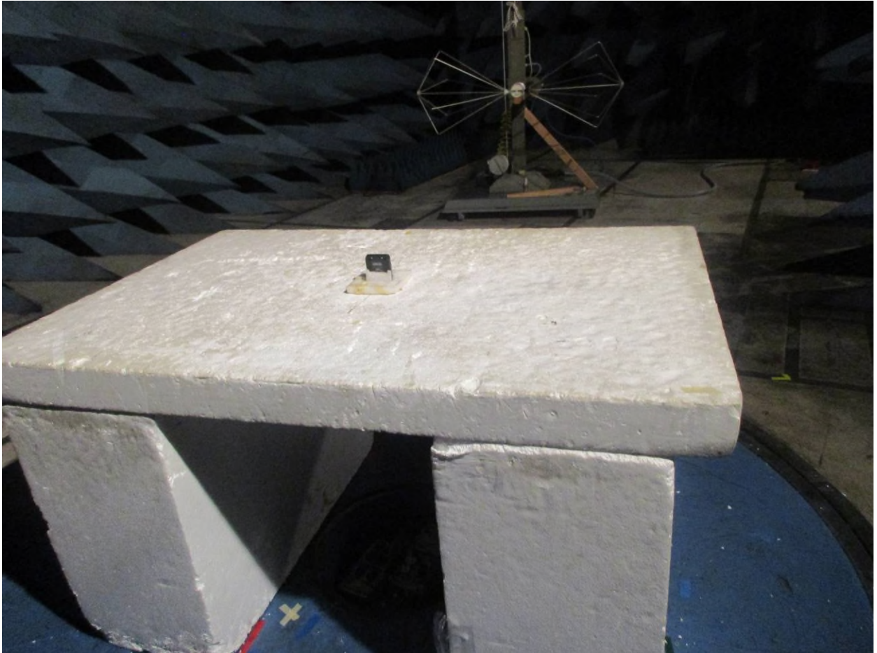
Figure 7: Radiated Emissions – Back View – EUT Standing (30 MHz – 200 MHz)
