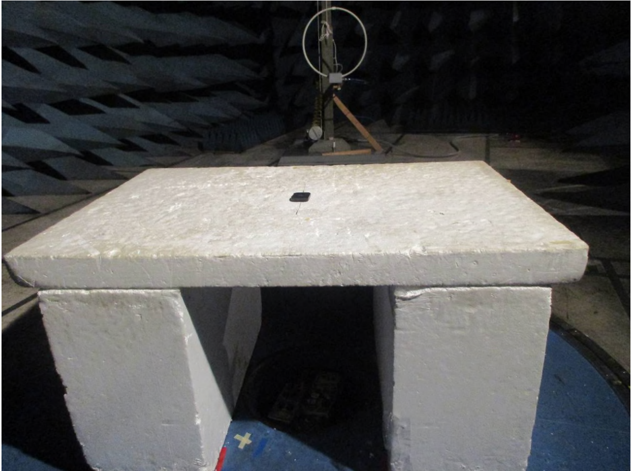
Figure 2: Radiated Emissions – Back View – EUT Flat (below 30 MHz)
