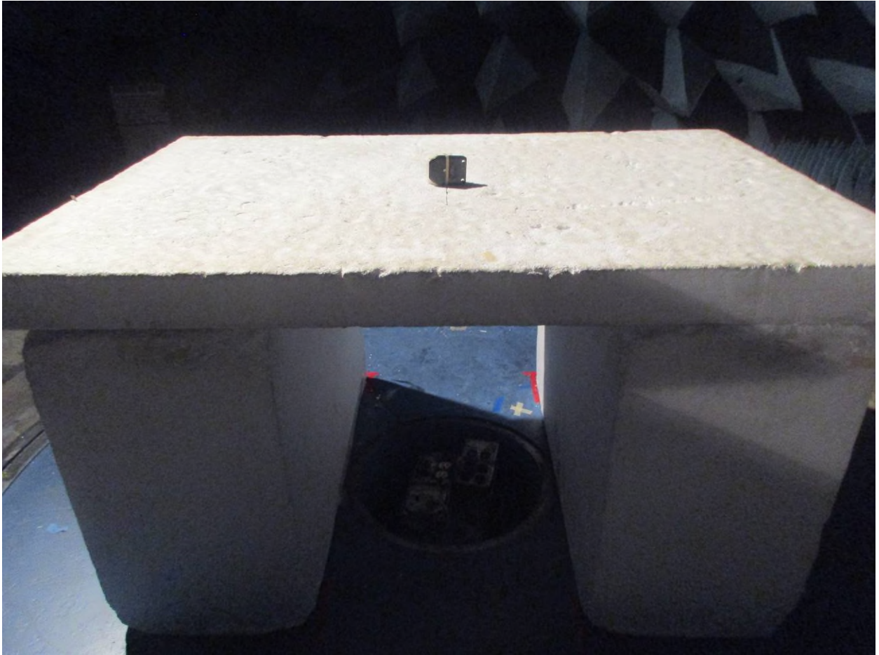
Figure 9: Radiated Emissions – Front View - EUT Sideways
