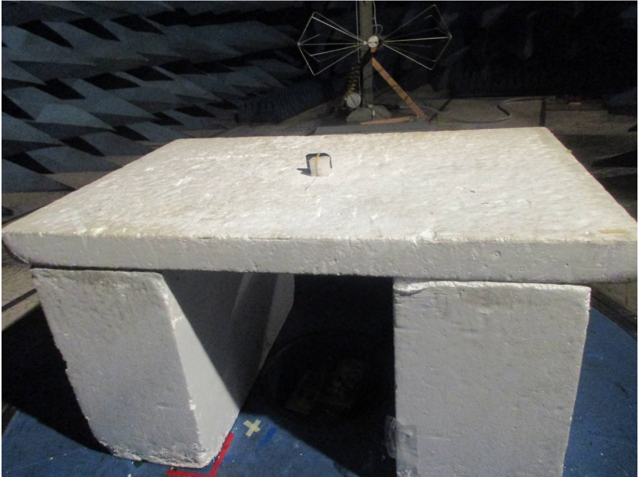
Figure 11: Radiated Emissions – Back View – EUT Sideways (30 MHz – 200 MHz)
