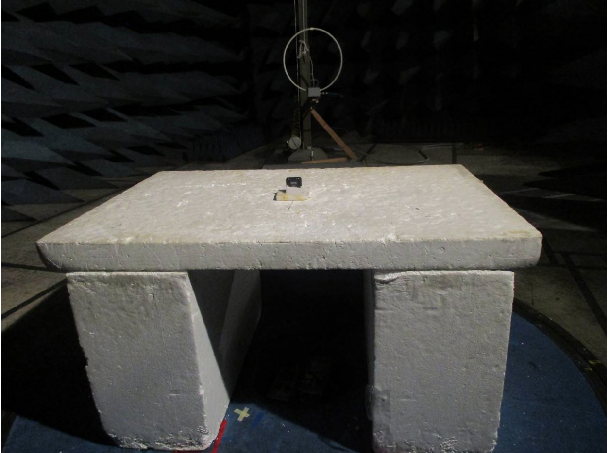
Figure 6: Radiated Emissions – Back View – EUT Standing (below 30 MHz)
