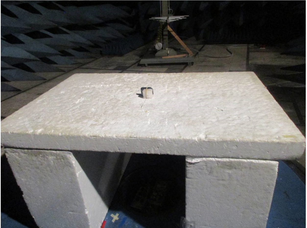
Figure 12: Radiated Emissions – Back View – EUT Sideways (200 MHz – 1 GHz)
