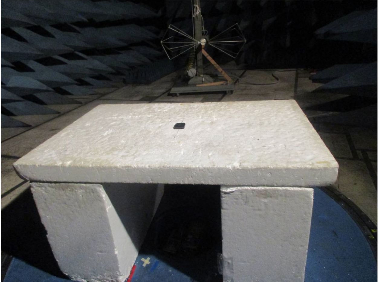
Figure 3: Radiated Emissions – Back View – EUT Flat (30 MHz – 200 MHz)
