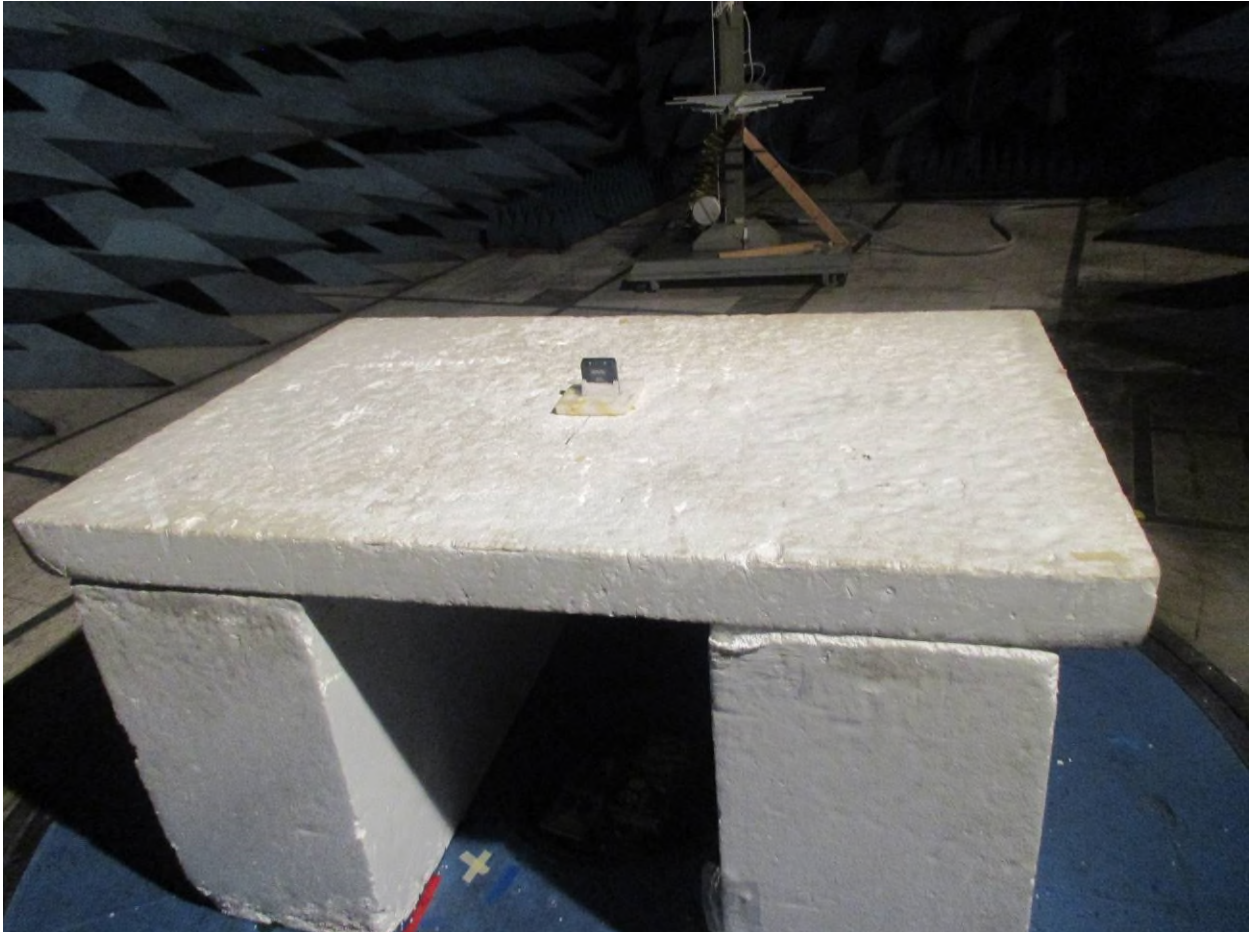
Figure 8: Radiated Emissions – Back View – EUT Standing (200 MHz – 1 GHz)
