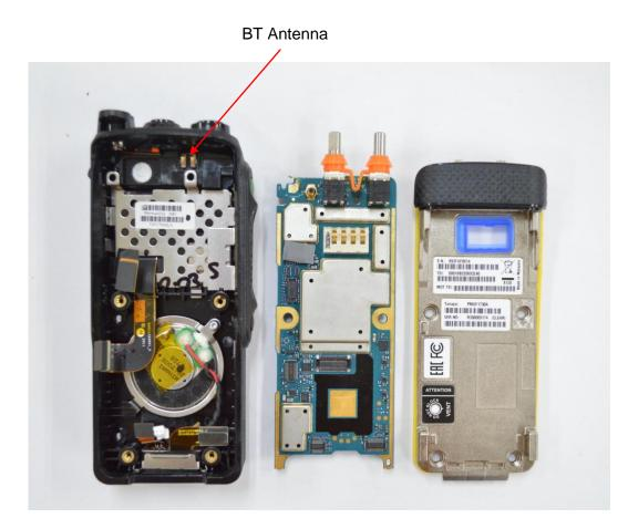
RF Board with Chassis and Housing (Back Side), Model MTP3550 / MTP3500
