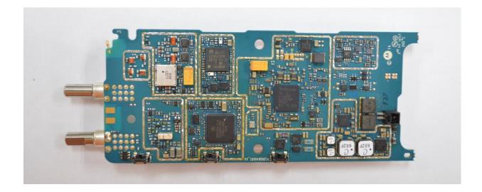
RF board without Shields (Top), Model MTP3550 / MTP3500
