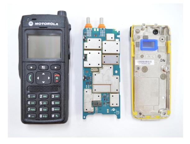
RF Board with Chassis and Housing (Front Side), Model MTP3550
