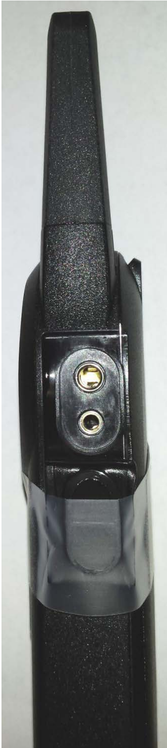
Side View (Accessory Jack) (DLR1020 and DLR1060)
