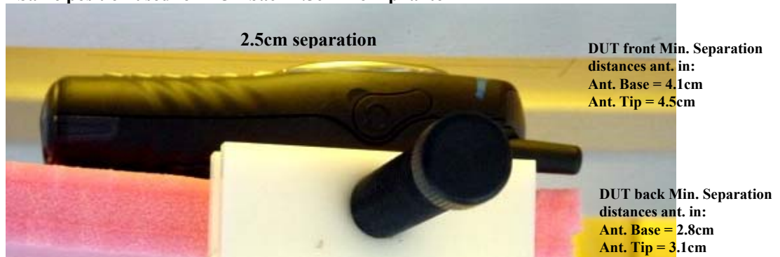
Figure 9: Robot Test System (Flat Phantom)
