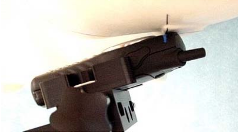
Figure 2. Assessment @ the Left ear; 15° tilt position; (DUT antenna retracted. Same position used for antenna extended.)
