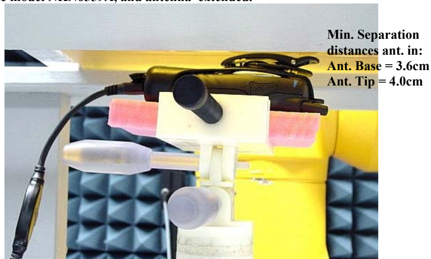
Figure 6. Assessment @ Abdomen; DUT w/ carry case model NNTN4755A against the flat phantom and attached data cable model NKN6560A. Same position used to assess data cable model NKN6559A, and antenna extended.
