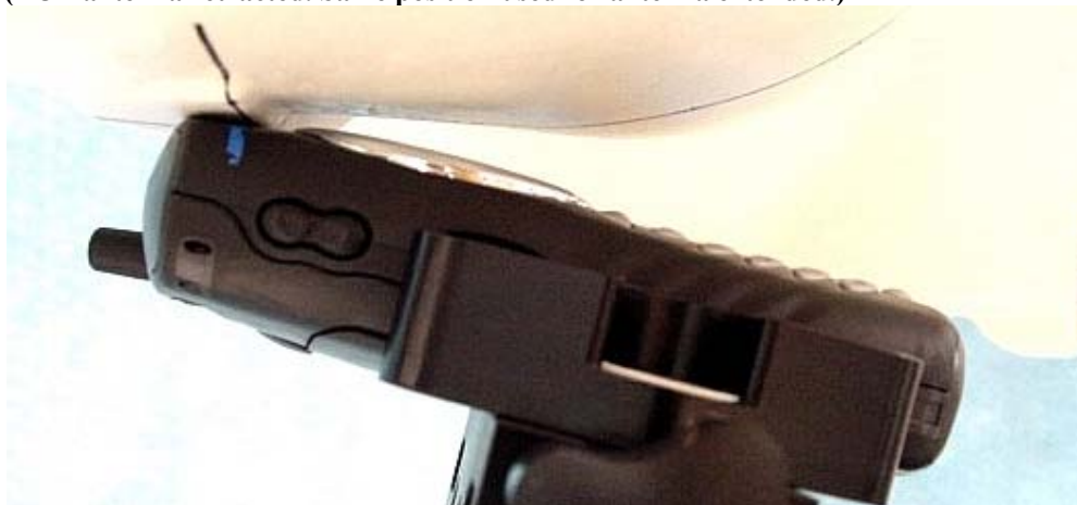
Figure 4. Assessment @ the Right ear; 15° tilt position; (DUT antenna retracted. Same position used for antenna extended.)
