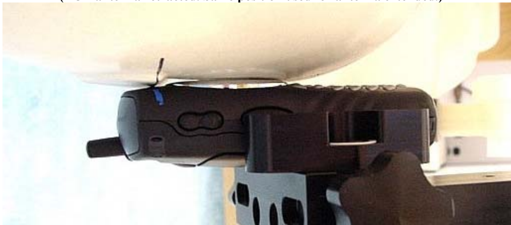
Figure 3. Assessment @ the Right ear; Cheek touch position; (DUT antenna retracted. Same position used for antenna extended.)
