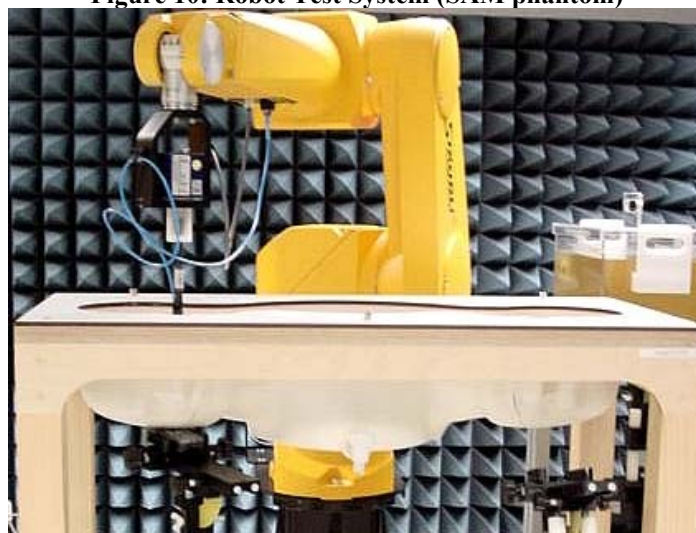
Figure 10: Robot Test System (SAM phantom)
