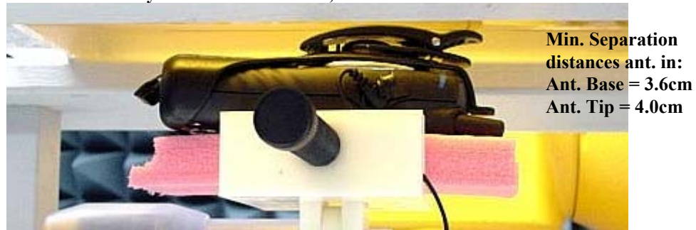
Figure 7. Assessment @ the Abdomen; with carry case model NNTN4755A and attached audio accessory model SYN8390B. Same position used to assess audio accessory models NNTN4033A, and NSN6066A w/ antenna in and out.
