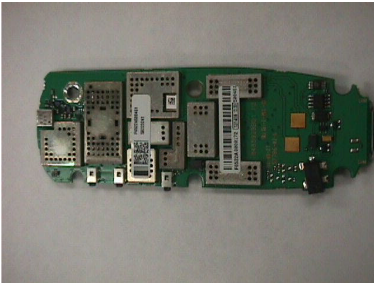
Photograph 9-2: Front side of radio main board .
