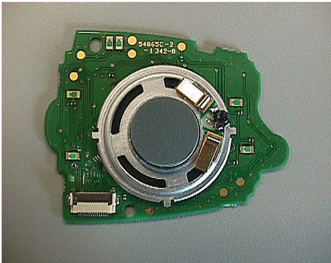
Photograph 9-5: Back side of keypad board, showing attached speaker.
