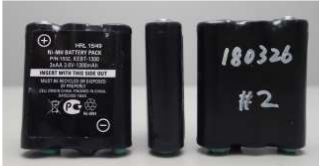
Battery 1532: Front, Side, Back View
