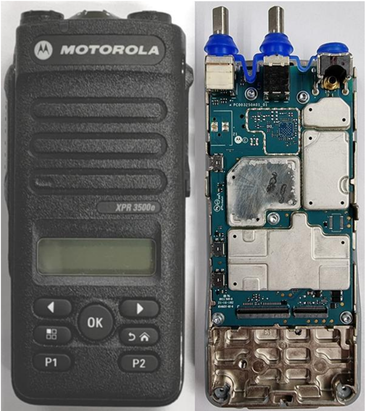
RF board with chassis and housing for Display and Limited Keypad model (front side) TIA4950
