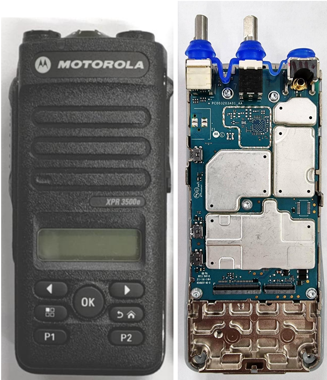
RF board with chassis and housing for Display and Limited Keypad model (front side) Non-TIA4950
