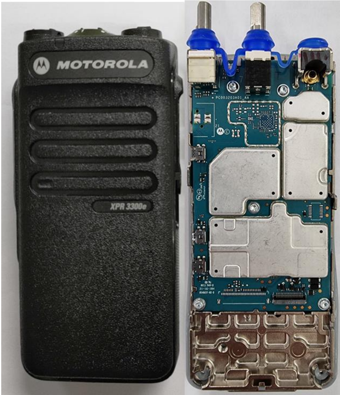
RF board with chassis and housing for Non Keypad model (front side) Non-TIA4950
