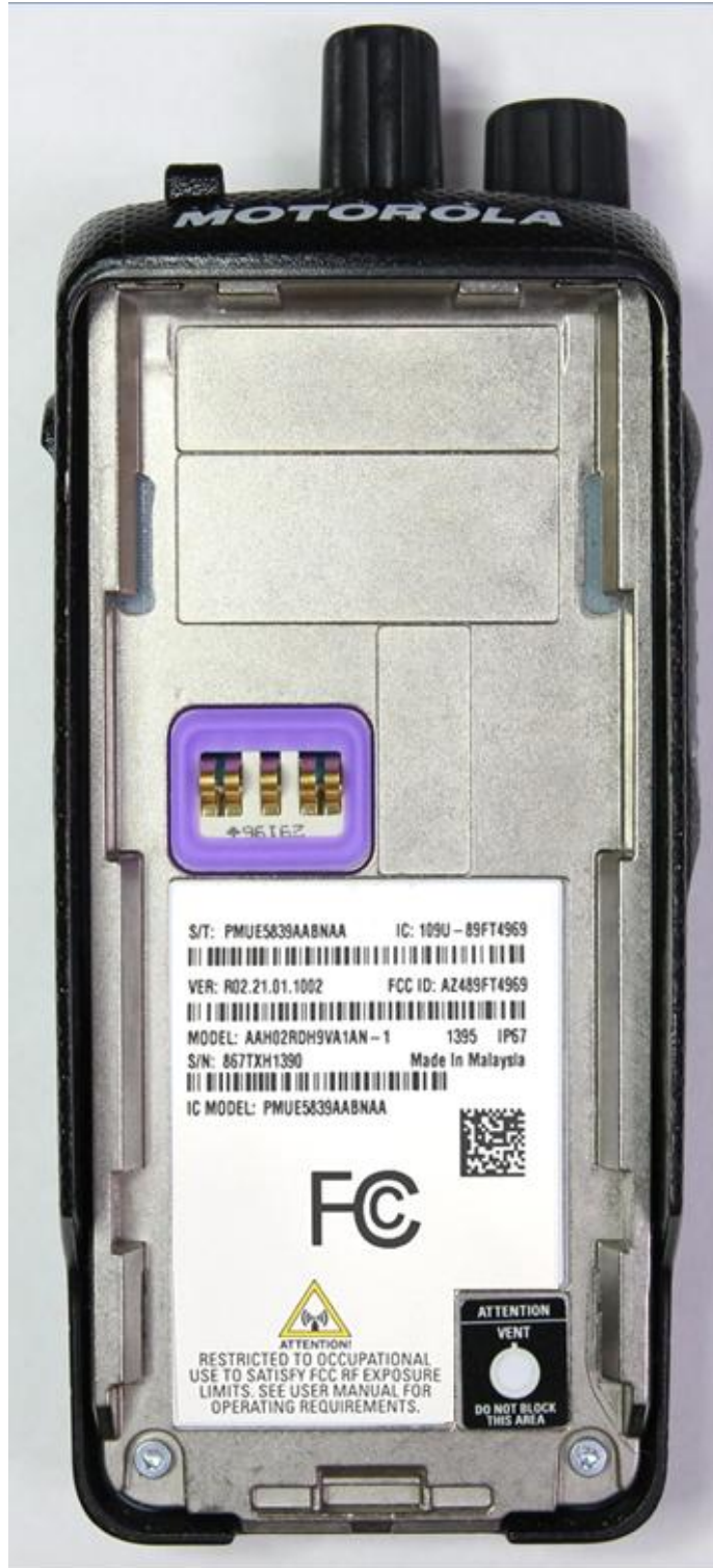
Back View for Limited Keypad and Plain Model (FCC/IC label) – XPR 3500e & XPR 3300e
