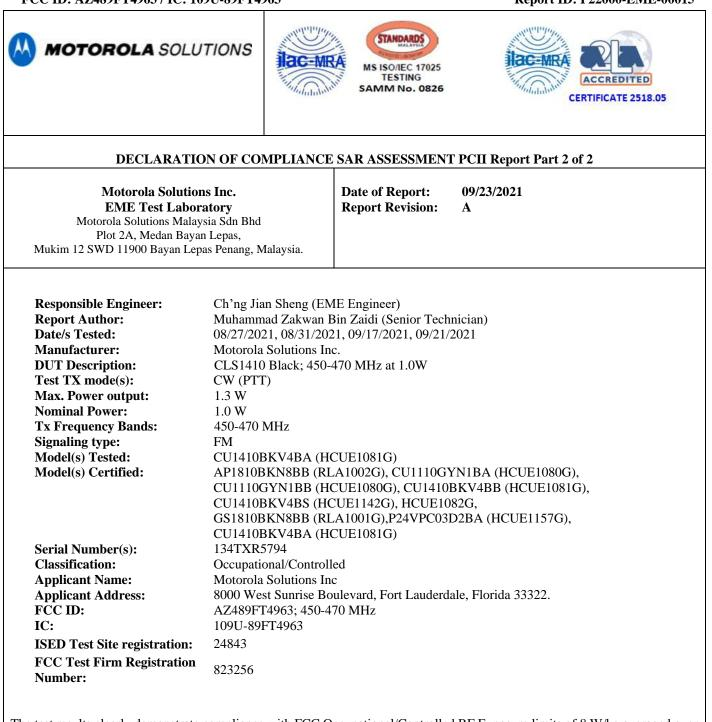
The test results clearly demonstrate compliance with FCC Occupational/Controlled RF Exposure limits of 8 W/kg averaged over 1 gram per the requirements of FCC 47 CFR § 2.1093 and RSS-102 (Issue 5).
