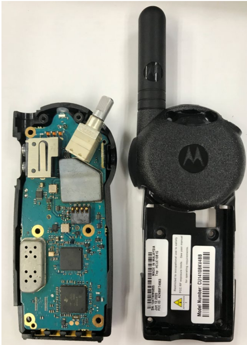
RF board with chassis and housing (Back Side) [CLS1410: CU1410BKV4BB]
