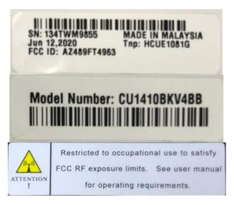
Figure 2: FCC Label for CU1410BKV4BB (CLS1410)
