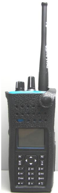
DUT Front View Hard Leather Carry Case w/ Swivel Belt Loop PMLN6097A 2.5 inch
