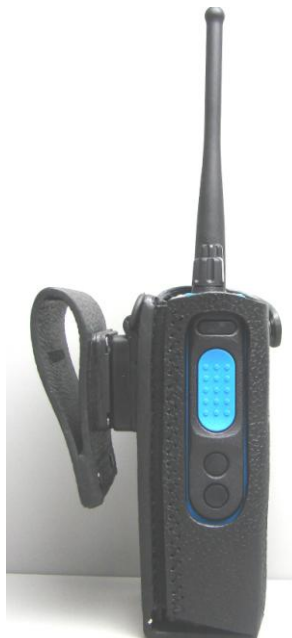
DUT Side View Hard Leather Carry Case w/ Swivel Belt Loop PMLN6097A 2.5 inch
