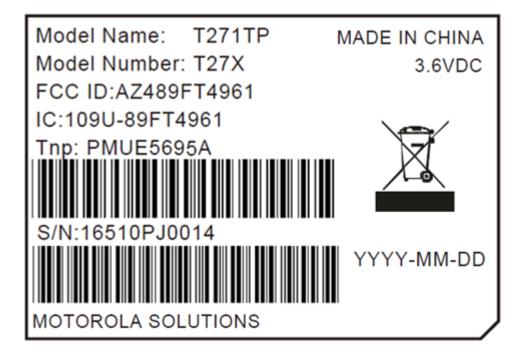
Figure 2: FCC/IC Label for T271TP
