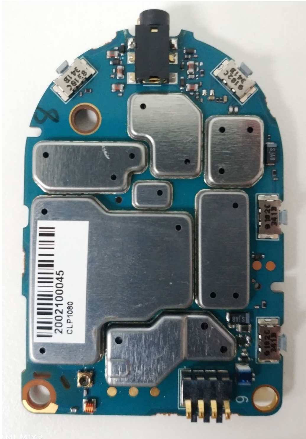
RF board with Shields (Bottom) (CLP1080e, CLP1083e, CLP1010e, CLP1013e)
