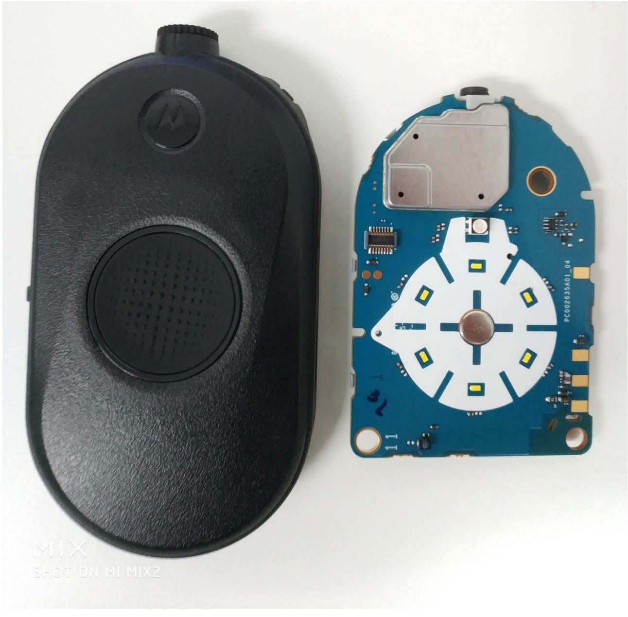
RF board with housing (front side) (CLP1080e, CLP1083e, CLP1010e, CLP1013e)
