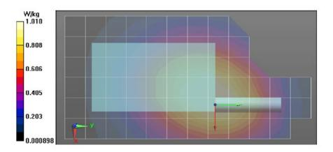
Shortened scan reflects highest SAR producing configuration and is compared to the full scan.
