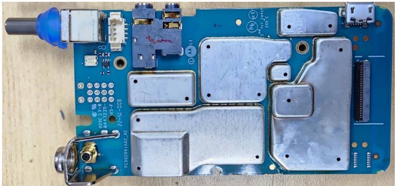
RF board with Shields (Bottom) of Limited Keypad (LKP) / Full Keypad (FKP) model AAH87YDH9JA2AN / AAH87YDF9JA2AN / AAH87YDH9JC2AN
