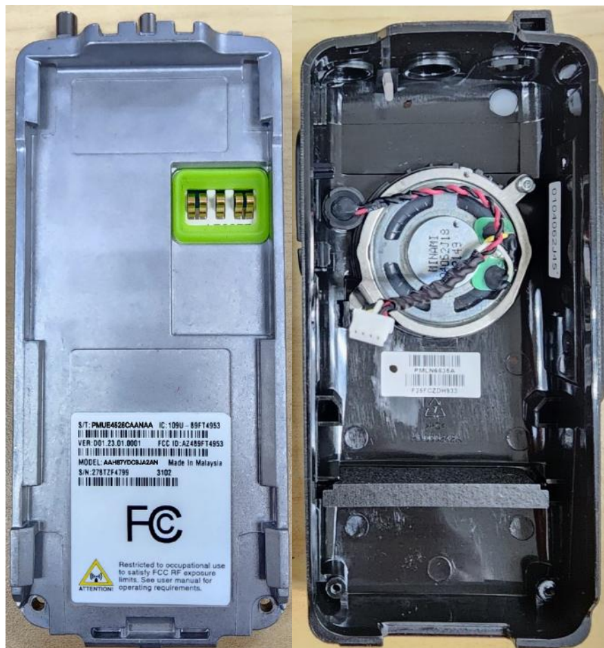
Chassis and Housing (Back side) of Non Keypad (NKP) model LAH87YDC9JA2AN / AAH87YDC9JA2AN / AAH87YDC9JC2AN
