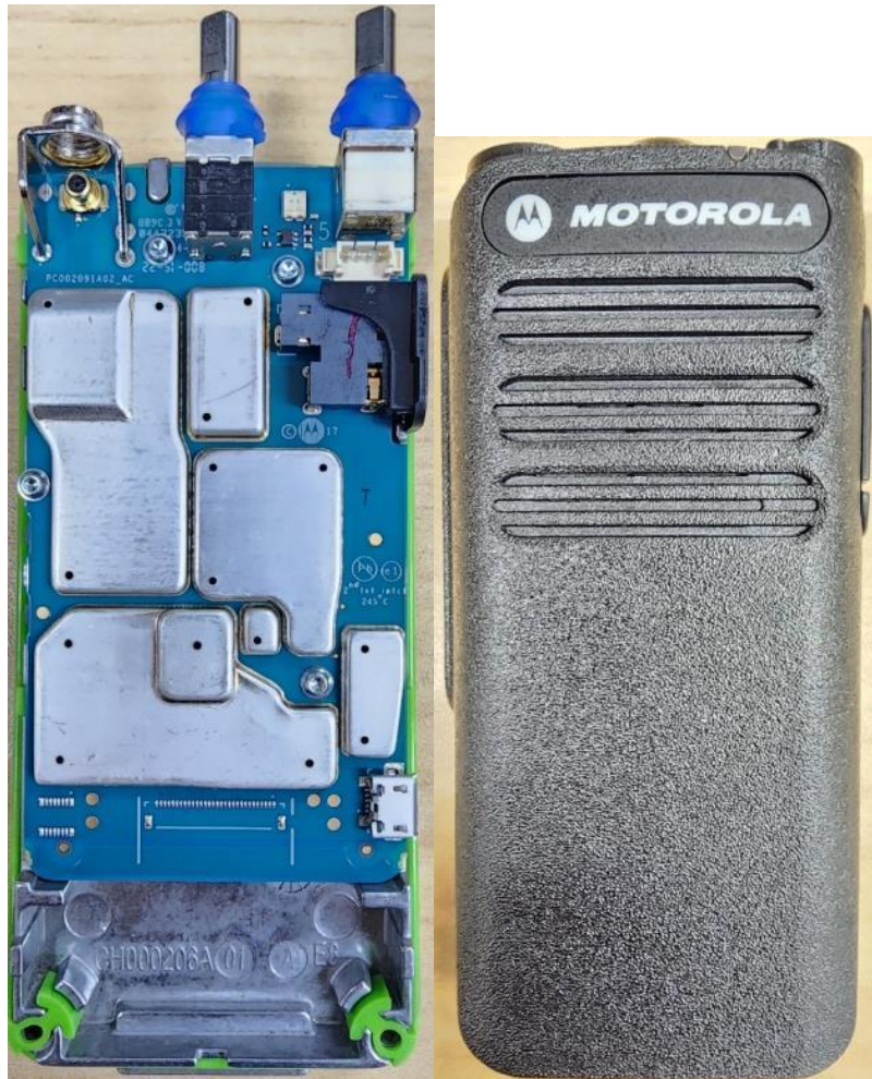
RF board with chassis and housing (front side) of Non Keypad (NKP) model LAH87YDC9JA2AN / AAH87YDC9JA2AN / AAH87YDC9JC2AN
