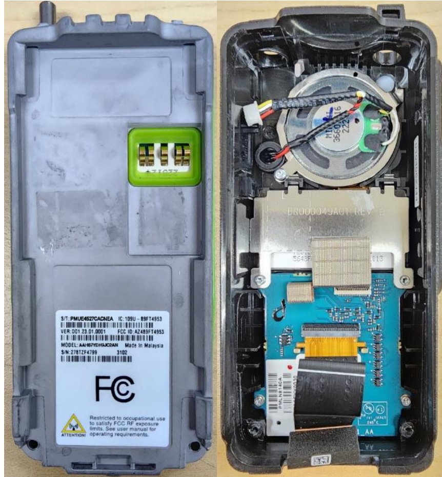
Chassis and Housing (Back side) of Limited Keypad (LKP) AAH87YDH9JC2AN
