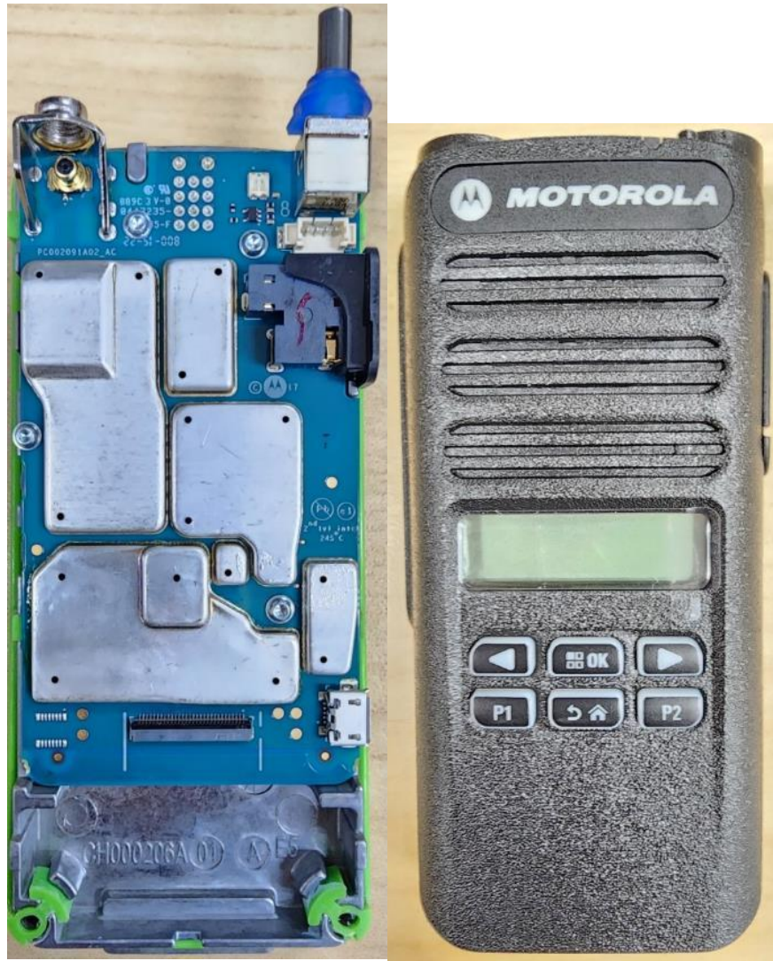
RF board with chassis and housing (front side) of Limited Keypad (LKP) model AAH87YDH9JA2AN / AAH87YDH9JC2AN
