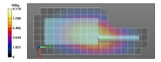
Shortened scan reflects highest SAR producing configuration and is compared to the full scan.
