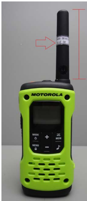
Antenna model: EAN.144F.823RA1 (pointed with arrow)
