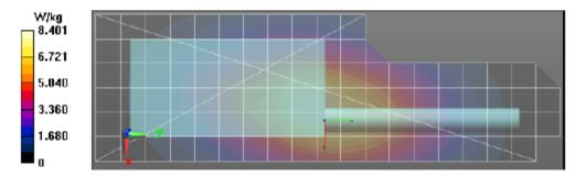
Shortened scan reflects highest SAR producing configuration and is compared to the full scan.
